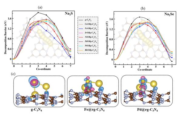
Fig. 5 Decomposition paths and decomposition energies of (a)  $Na_2S$  and (b)  $Na_2S$  on the pristine  $g-C_3N_4$  and  $SA@rg-C_3N_4$  monolayers. (c) The charge density differences of  $Na_2S$  adsorbed on the pristine  $g-C_3N_4$  and  $SA@rg-C_3N_4$  monolayer. The blue regions represent electron accumulation, and magenta regions represent depletion.
