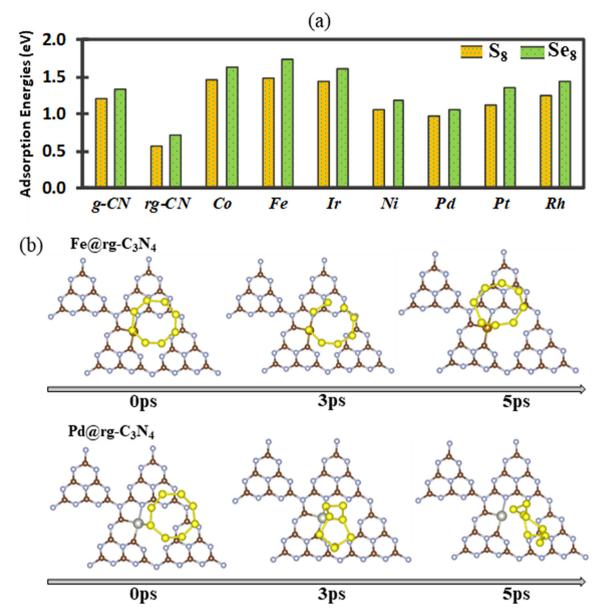
Fig. 2 (a) The adsorption energies of  $X_8$  (X = S and Se) adsorbed on the surface of pristine, reduced g- $C_3N_4$ , and SA@rg- $C_3N_4$  (SA = Co, Fe, Ir, Ni, Pd, Pt, and Rh). (b) Snapshot at 5 ps of AIMD simulations of the adsorption of  $S_8$  on SA@rg-C<sub>3</sub>N<sub>4</sub> for SA = Fe and Pd.
