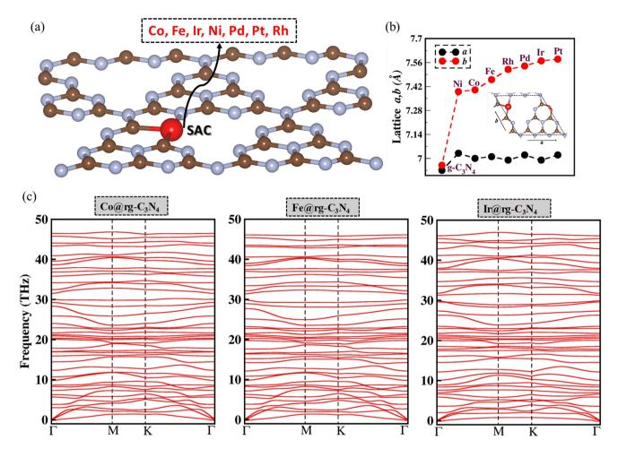
Fig. 1 (a) Perspective view of a SA adsorbed on the  $rg-C_3N_4$  support. (b) Lattice constant of the SA@rg-C<sub>3</sub>N<sub>4</sub> monolayer for a 1 × 1 unit cell as represented in the inset. (c) Phonon spectra curves of SA@rg-C<sub>3</sub>N<sub>4</sub> for SA = Co, Fe, Ir.
