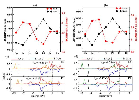
Fig. 6 The strength of (a) Na-S and SA-S bonds and (b) Na-Se and SA-Se evaluated using the integrated COHP (-ICOHP) for the Na<sub>2</sub>X-SAC system. (Here, the depicted bond strength (-ICOHP) is the sum of the spin-up and spin-down -ICOHP values in eV per bond.) (c and d) The calculated partial density of states (PDOS) of Na<sub>2</sub>X-SAC (SAC = Fe, Pd) systems. The up-spin d-band center values are illustrated on the PDOS plot, measured with respect to the Fermi level set at zero.
