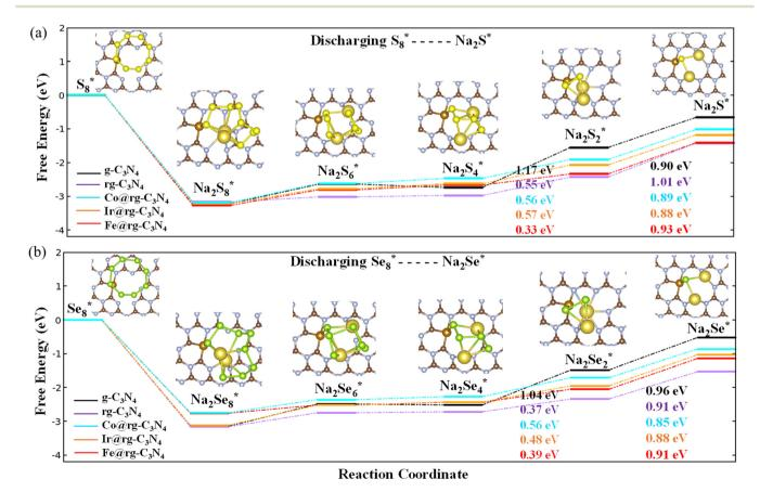
Fig. 4 Energy profiles for the reduction of (a) Na-pSs and (b) Na-pSes on  $g-C_3N_4$ ,  $rg-C_3N_4$  and SA@rg-C<sub>3</sub>N<sub>4</sub> (SA = Co, Fe, Ir) monolayer. The inset images are the top view of Na-pXs adsorbed on the substrates.
