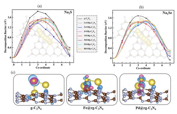
Fig. 5 Decomposition paths and decomposition energies of (a) Na<sub>2</sub>S and (b) Na<sub>2</sub>Se on the pristine g-C<sub>3</sub>N<sub>4</sub> and SA@rg-C<sub>3</sub>N<sub>4</sub> monolayers. (c) The charge density differences of Na<sub>2</sub>S adsorbed on the pristine g-C<sub>3</sub>N<sub>4</sub> and SA@rg-C<sub>3</sub>N<sub>4</sub> monolayer. The blue regions represent electron accumulation, and magenta regions represent depletion.
