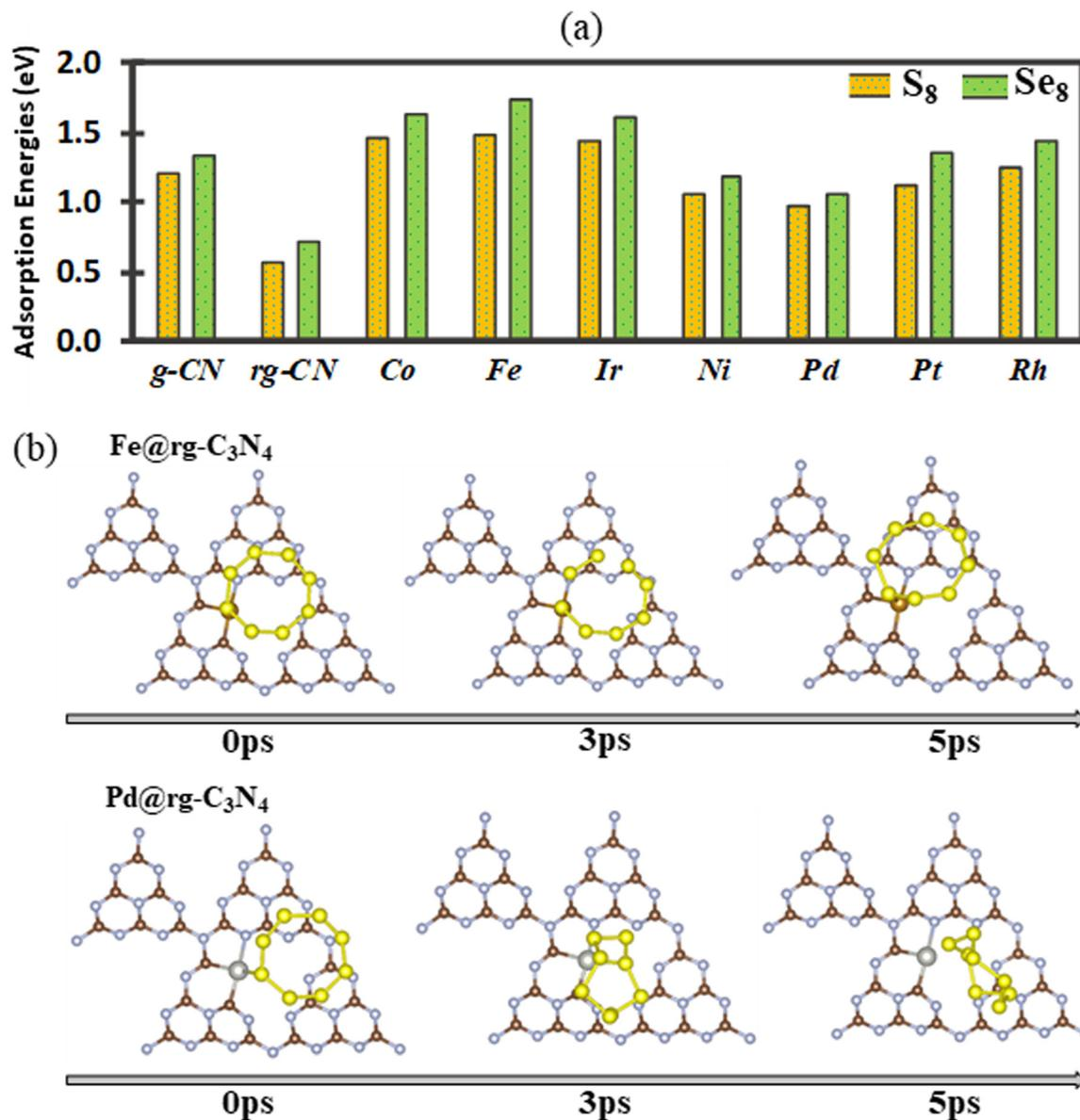
**Fig. 2** (a) The adsorption energies of  $X_8$  ( $X = S$  and  $Se$ ) adsorbed on the surface of pristine, reduced  $g-C_3N_4$ , and  $SA@rg-C_3N_4$  ( $SA = Co, Fe, Ir, Ni, Pd, Pt,$  and  $Rh$ ). (b) Snapshot at 5 ps of AIMD simulations of the adsorption of  $S_8$  on  $SA@rg-C_3N_4$  for  $SA = Fe$  and  $Pd$ .
