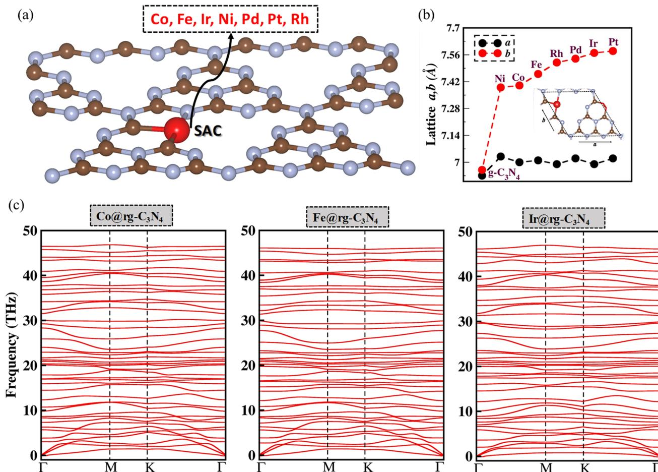
Fig. 1 (a) Perspective view of a SA adsorbed on the rg-C<sub>3</sub>N<sub>4</sub> support. (b) Lattice constant of the SA@rg-C<sub>3</sub>N<sub>4</sub> monolayer for a 1 × 1 unit cell as represented in the inset. (c) Phonon spectra curves of SA@rg-C<sub>3</sub>N<sub>4</sub> for SA = Co, Fe, Ir.
