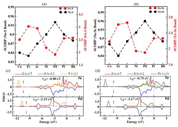
Fig. 6 The strength of (a) Na-S and SA-S bonds and (b) Na-Se and SA-Se evaluated using the integrated COHP (-ICOHP) for the  $Na_2X-SAC$ system. (Here, the depicted bond strength (-ICOHP) is the sum of the spin-up and spin-down -ICOHP values in eV per bond.) (c and d) The calculated partial density of states (PDOS) of Na<sub>2</sub>X-SAC (SAC = Fe, Pd) systems. The up-spin d-band center values are illustrated on the PDOS plot, measured with respect to the Fermi level set at zero.
