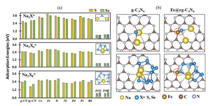
Fig. 3 (a) The adsorption energies of  $Na_2X_n$  (n = 1, 4, 8) adsorbed on SA@rg- $C_3N_4$ . (b) Geometrical structures of  $Na_2X_n$  (n = 1, 8) adsorbed on a pristing  $g-C_3N_4$  and Fe@rg- $C_3N_4$  monolayer.
