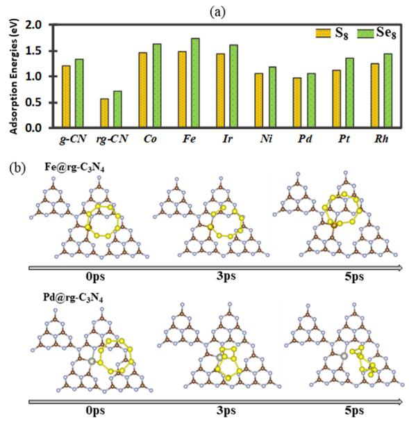
Fig. 2 (a) The adsorption energies of  $X_8$  (X = S and Se) adsorbed on the surface of pristine, reduced g- $C_3N_4$ , and SA@rg- $C_3N_4$  (SA = Co, Fe, Ir, Ni, Pd, Pt, and Rh). (b) Snapshot at 5 ps of AIMD simulations of the adsorption of  $S_8$  on SA@rg-C<sub>3</sub>N<sub>4</sub> for SA = Fe and Pd.
