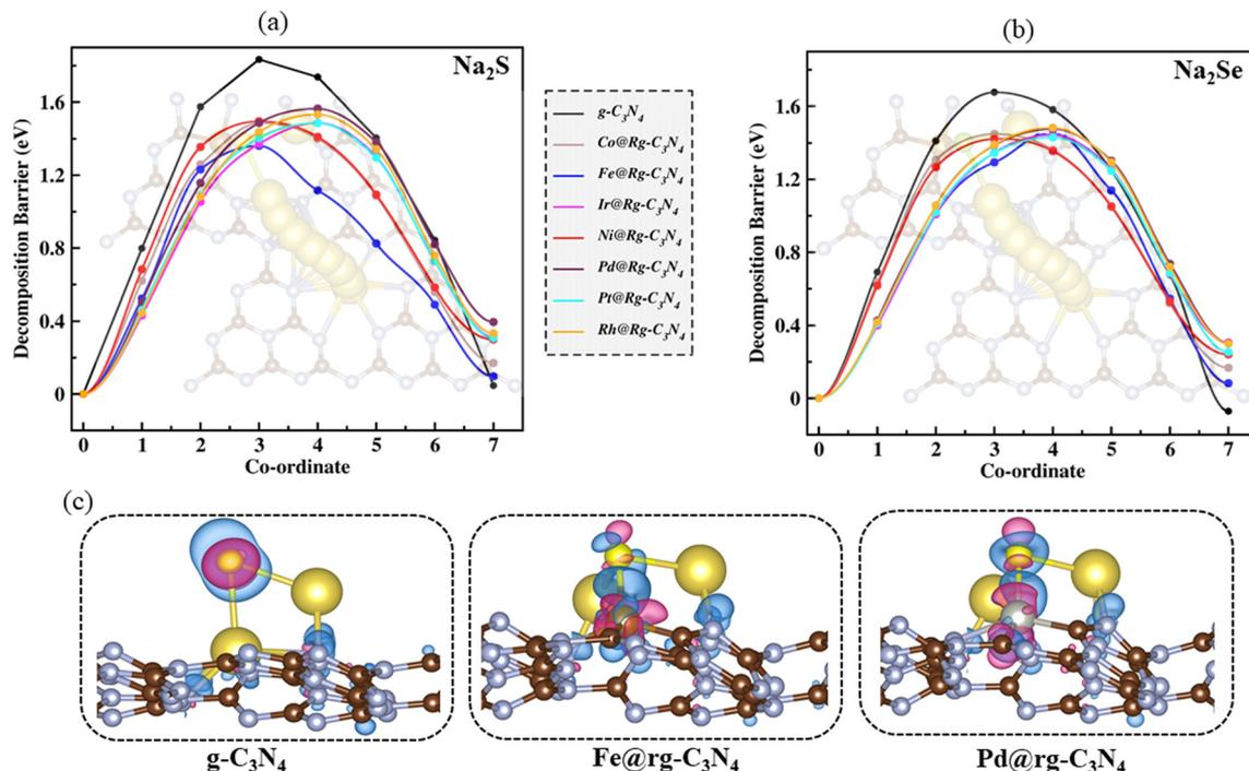
Fig. 5 Decomposition paths and decomposition energies of (a) Na<sub>2</sub>S and (b) Na<sub>2</sub>Se on the pristine g-C<sub>3</sub>N<sub>4</sub> and SA@rg-C<sub>3</sub>N<sub>4</sub> monolayers. (c) The charge density differences of Na<sub>2</sub>S adsorbed on the pristine g-C<sub>3</sub>N<sub>4</sub> and SA@rg-C<sub>3</sub>N<sub>4</sub> monolayer. The blue regions represent electron accumulation, and magenta regions represent depletion.
