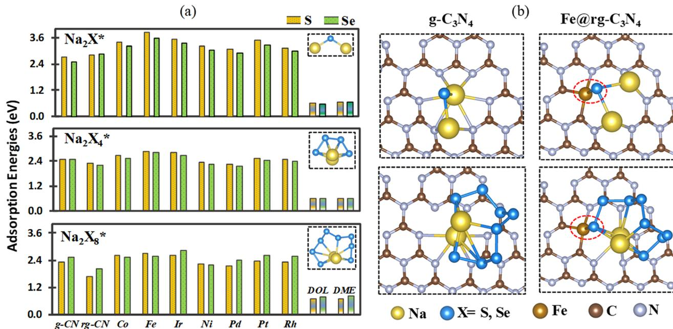
Fig. 3 (a) The adsorption energies of Na<sub>2</sub>X<sub>n</sub> ( $n = 1, 4, 8$ ) adsorbed on SA@rg-C<sub>3</sub>N<sub>4</sub>. (b) Geometrical structures of Na<sub>2</sub>X<sub>n</sub> ( $n = 1, 8$ ) adsorbed on a pristine g-C<sub>3</sub>N<sub>4</sub> and Fe@rg-C<sub>3</sub>N<sub>4</sub> monolayer.
