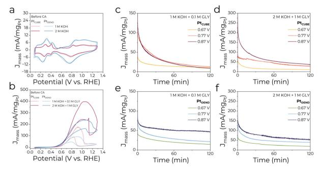
Fig. 2 CV profiles of Pt nanocatalysts in (a) 1 M KOH and 2 M KOH and (b) 1 M KOH + 0.1 M GLY and 2 M KOH + 1 M GLY electrolytes. Potentiostatic electrolysis at 0.67, 0.77 and 0.87 V for (c and d) Pt<sub>CUBE</sub> and (e and f) Pt<sub>DEND</sub> in 1 M KOH + 0.1 M GLY and 2 M KOH + 1 M GLY electrolytes. The currents are normalised by the absolute Pt mass loading.
