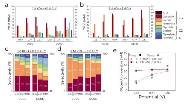
Fig. 3 The yields of GEOR products after 2 hours of electrolysis at 0.67, 0.77 and 0.87 V and selectivity of GEOR products performed in (a and c) 1 M KOH + 0.1 M GLY and (b and d) 2 M KOH + 1 M GLY electrolytes. (e) Glycerol conversion in 1 M KOH + 0.1 M GLY and 2 M KOH + 1 M GLY electrolytes. Note that in (c and d), the selectivity of products less than or equal to 3% is not marked.
