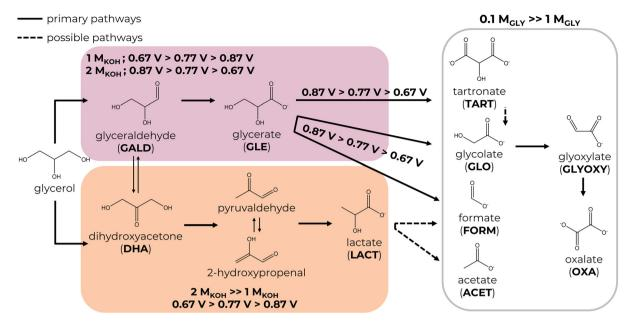
Scheme 2 Proposed GEOR mechanism on the Pt<sub>NPs</sub>/CFP electrodes in an alkaline medium.
