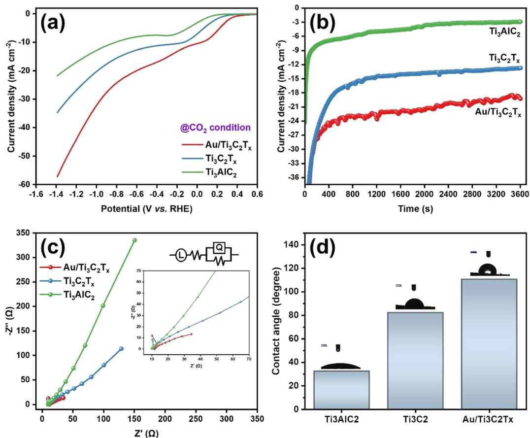
**Fig. 6** Assessment of the electrocatalytic efficiency of catalysts composed of  $\text{Ti}_3\text{AlC}_2$ ,  $\text{Ti}_3\text{C}_2\text{T}_x$  and  $\text{Au}/\text{Ti}_3\text{C}_2\text{T}_x$  in the ECRR: (a) LSV plots; (b) chronoamperometric responses at  $-0.62$  V vs. RHE; (c) EIS conducted on  $\text{Au}/\text{Ti}_3\text{C}_2\text{T}_x$ ,  $\text{Ti}_3\text{C}_2\text{T}_x$ , and  $\text{Ti}_3\text{AlC}_2$ . Inset: equivalent electrical circuit; and (d) contact angle.
