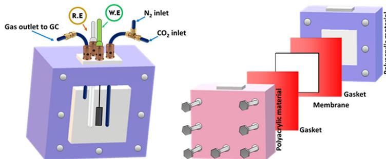
Fig. 5 Electrochemical cell used in the ECRR experiment.
