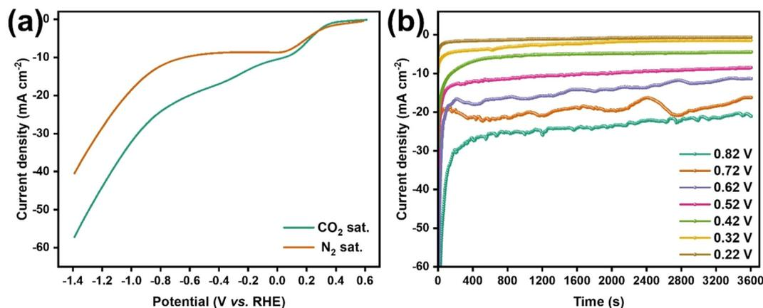
Fig. 7 Electrochemical activity of the Au/Ti<sub>3</sub>C<sub>2</sub>T<sub>x</sub> composites for the ECRR. (a) LSVs under CO<sub>2</sub> saturated and N<sub>2</sub> saturated conditions and (b) chronoamperometric curves at a potential of  $-0.22$  V (brown) and  $-0.82$  V (green) vs. RHE (colour on line).
