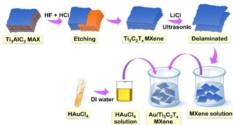
Fig. 1 Schematic illustration of the preparation of Au/Ti<sub>3</sub>C<sub>2</sub>T<sub>x</sub>.
