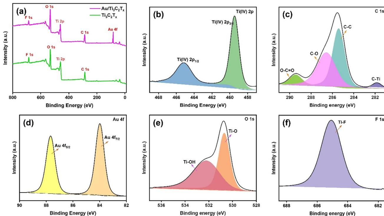
Fig. 3 (a) The full survey XPS spectrum, and (b) Ti 2p, (c) C 1s, (d) Au 4f, (e) O 1s and (f) F 1s spectra of  $\text{Au}/\text{Ti}_3\text{C}_2\text{T}_x$ .
