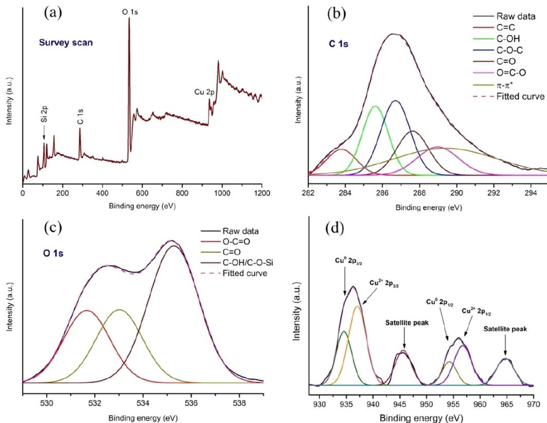
Fig. 7 XPS analysis of the Cu-CuO@rGO-SiO<sub>2</sub> nanocomposite. Survey scan (a), high resolution C 1s (b), high resolution O 1s (c), and high resolution Cu 2p (d).
