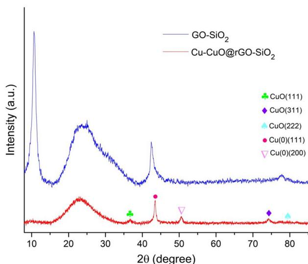
Fig. 2 XRD patterns of GO-SiO<sub>2</sub> and Cu-CuO@rGO-SiO<sub>2</sub>.
