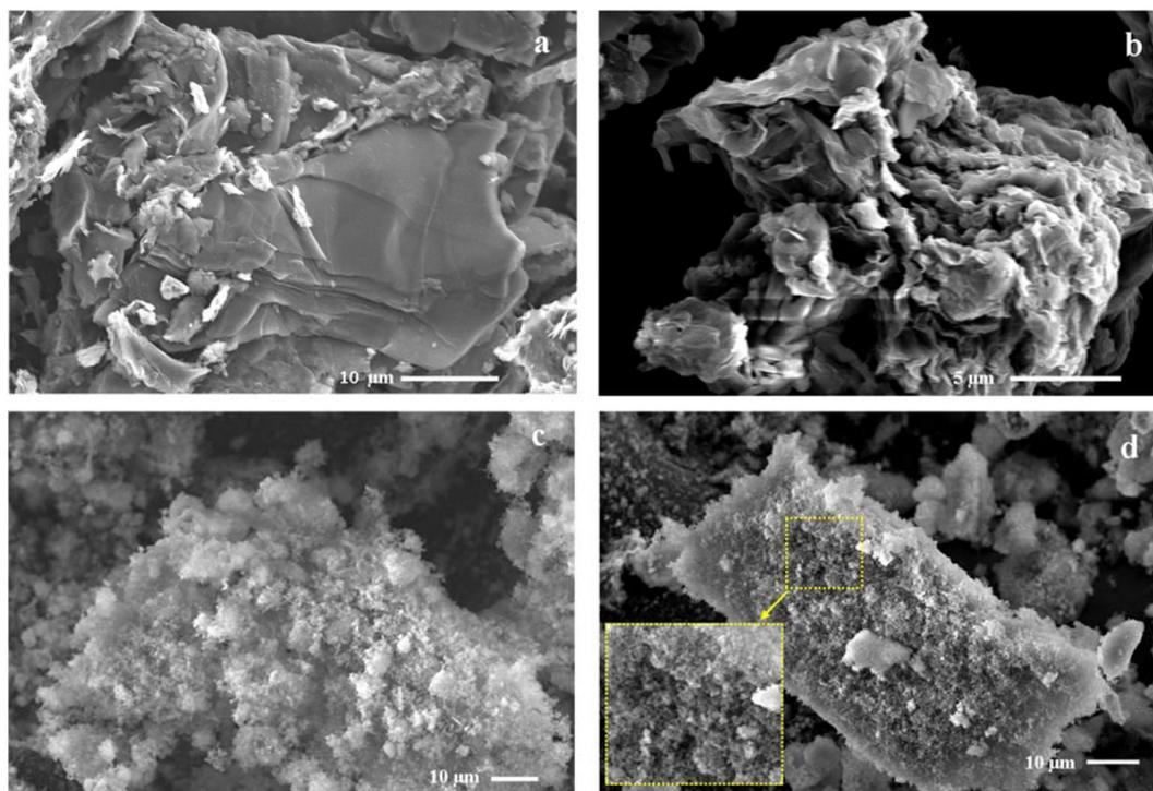
Fig. 4 SEM images of (a) graphite, (b) graphene oxide, (c) the GO-SiO<sub>2</sub> hybrid, and (d) Cu-CuO@rGO-SiO<sub>2</sub>.
