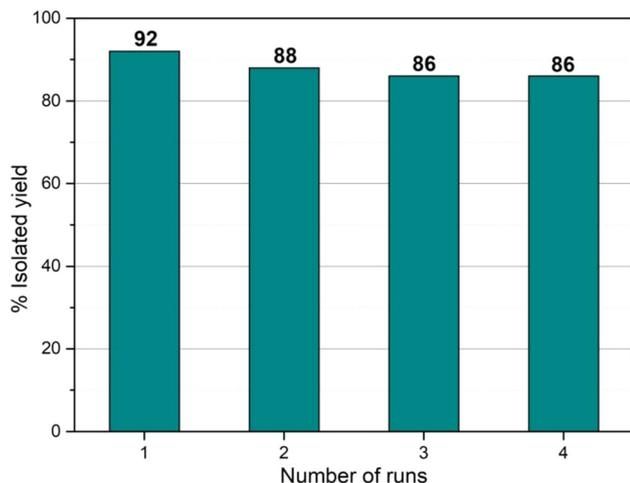
**Fig. 10** Recyclability of the Cu-CuO@rGO-SiO<sub>2</sub> nanocomposite in the C-S cross-coupling reaction.
