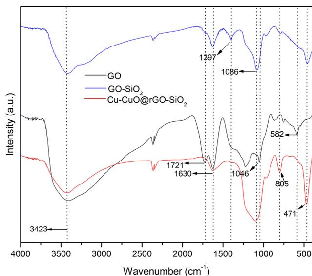
Fig. 1 FT-IR spectra of GO, GO-SiO<sub>2</sub> and Cu-CuO@rGO-SiO<sub>2</sub>.
