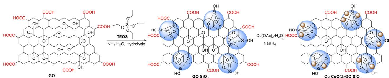
Scheme 1 Schematic representation of the synthesis of the Cu-CuO@rGO-SiO<sub>2</sub> nanocomposite.
