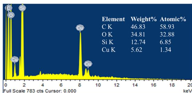
Fig. 5 SEM-EDS image of Cu-CuO@rGO-SiO<sub>2</sub>.
