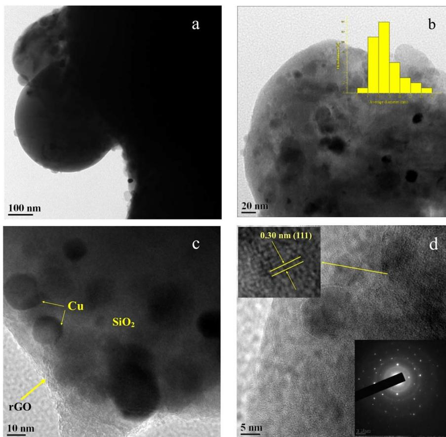
Fig. 6 HRTEM images of Cu-CuO@rGO-SiO<sub>2</sub> (a–c) and SAED patterns (d).
