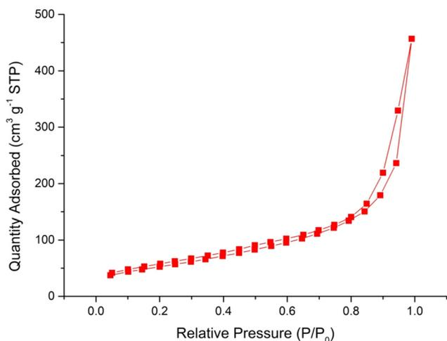
Fig. 8 BET analysis of the surface area of the Cu-CuO@rGO-SiO<sub>2</sub> nanocomposite.
