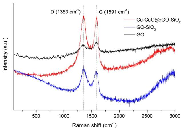
Fig. 3 Raman spectra of GO, GO-SiO<sub>2</sub> and Cu-CuO@rGO-SiO<sub>2</sub>.
