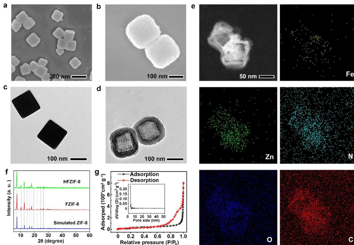
**Fig. 1** SEM images of the Fe-doped ZIF-8 (a) and HFZIF-8 (b). TEM images of the Fe-doped ZIF-8 (c), and HFZIF-8 (d). HAADF-STEM image and EDS element mappings of Fe, Zn, N, O, and C (e). XRD patterns of the Fe-doped ZIF-8, HFZIF-8, and simulated cards of ZIF-8 (f).  $N_2$  absorption–desorption isotherm and corresponding pore-size distribution for HFZIF-8 (g).
