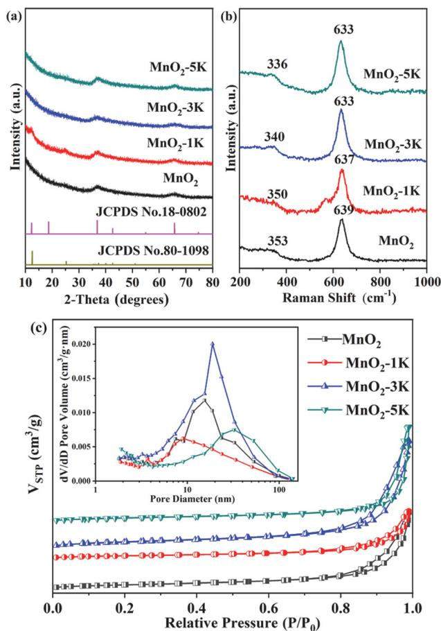
**Fig. 2** (a) XRD patterns and (b) Raman spectra of the prepared samples. (c) N<sub>2</sub> adsorption–desorption isotherms measured for the samples; the inset shows the corresponding pore size distribution curves.
