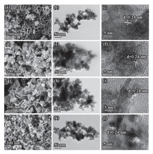
Fig. 3 SEM, TEM, and HR-TEM images (from left to right) of (a-c) MnO<sub>2</sub>, (d-f) MnO<sub>2</sub>-1K, (g-i) MnO<sub>2</sub>-3K, and (j-l) MnO<sub>2</sub>-5K.
