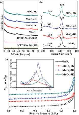
Fig. 2 (a) XRD patterns and (b) Raman spectra of the prepared samples. (c) N<sub>2</sub> adsorption-desorption isotherms measured for the samples; the inset shows the corresponding pore size distribution curves.
