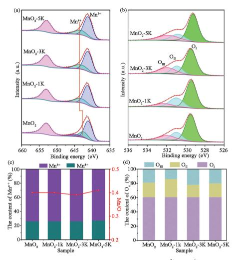
Fig. 4 (a) Mn 2p and (b) O 1s regions of the XPS spectra of four samples. (c) The content of Mn<sup>3+</sup> and Mn<sup>4+</sup> and the ratio of Mn/O. (d) The content of oxygen species.
