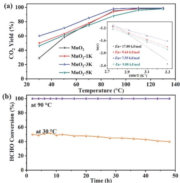
**Fig. 1** (a) Removal efficiency of HCHO on different catalysts with varying temperatures; the inset shows Arrhenius plots for the samples. (b) Stability of HCHO oxidation on MnO<sub>2</sub>-3K for 48 h at 30 °C and 90 °C. Reaction conditions: 500 ppm HCHO, 20 vol% O<sub>2</sub>, RH = 70%, GHSV = 60 000 mL (g h)<sup>-1</sup>.
