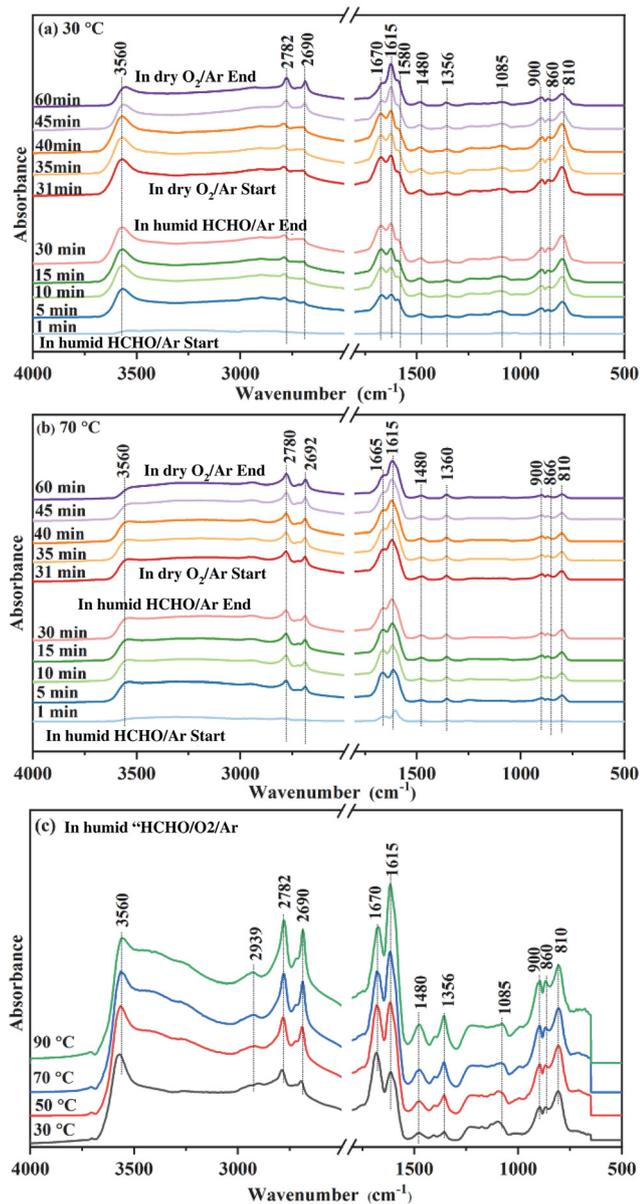
**Fig. 6** *In situ* DRIFTS of MnO<sub>2</sub>-3K, which was *in situ* heated in Ar at 400 °C for 30 min then cooled to 30 °C (a) and 70 °C (b). Humid HCHO/Ar was first introduced for 30 min, followed by dry O<sub>2</sub>/Ar for 30 min. (c) *In situ* DRIFTS of MnO<sub>2</sub>-3K at different temperatures under a flow of humid HCHO/O<sub>2</sub>/Ar. Each temperature was scanned for 10 min.
