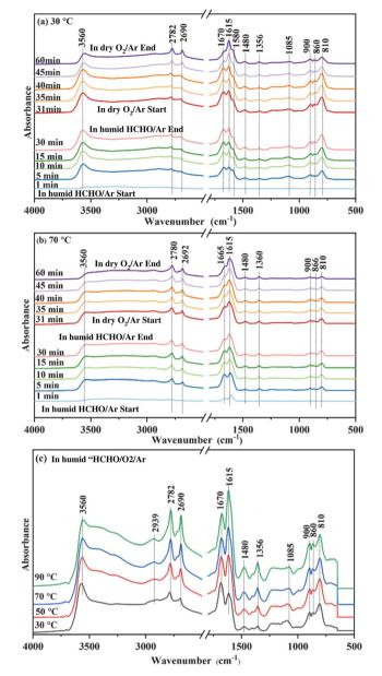
Fig. 6 In situ DRIFTS of MnO<sub>2</sub>-3K, which was in situ heated in Ar at 400 °C for 30 min then cooled to 30 °C (a) and 70 °C (b). Humid HCHO/Ar was first introduced for 30 min, followed by dry O<sub>2</sub>/Ar for 30 min. (c) In situ DRIFTS of MnO<sub>2</sub>-3K at different temperatures under a flow of humid HCHO/O<sub>2</sub>/Ar. Each temperature was scanned for 10 min.
