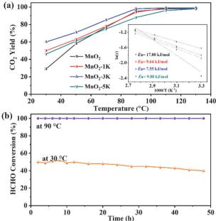
Fig. 1 (a) Removal efficiency of HCHO on different catalysts with varying temperatures; the inset shows Arrhenius plots for the samples. (b) Stability of HCHO oxidation on MnO<sub>2</sub>-3K for 48 h at 30 °C and 90 °C. Reaction conditions: 500 ppm HCHO, 20 vol% O2, RH = 70%, GHSV = 60 000 mL (g h)<sup>-1</sup>.
