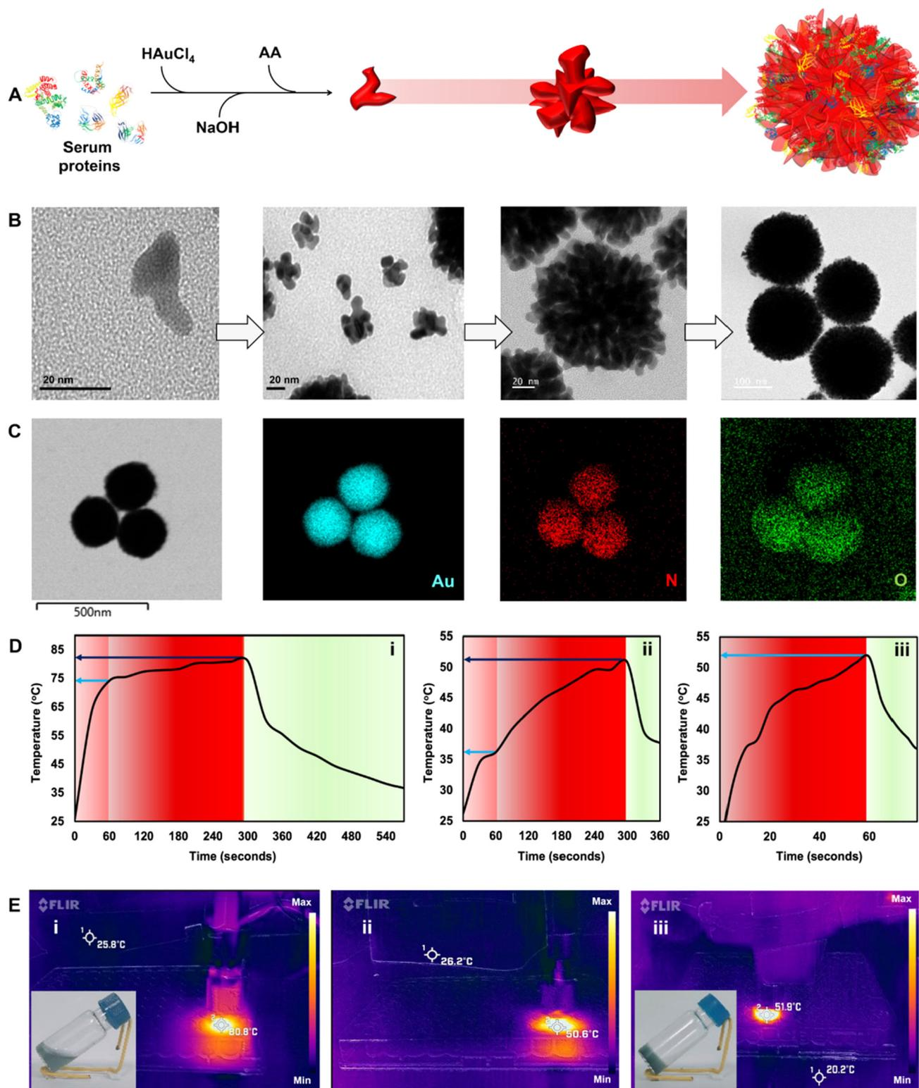
**Fig. 3** Characterization of plasmonic NanoSera (PNS). (A) Schematic of PNS formation; (B) different stages of PNS growth; (C) elemental mapping of PNS; (D) heating (red)–cooling (green) plots and (E) corresponding thermal images of PNS (i) in water, (ii) in Reliseal® and (iii) in PRP fibrin glue under 980 nm irradiation (dark blue and white arrows indicate the temperature at 300 and 60 seconds, respectively). Inset images show PNS (i) in water and (iii) in PRP fibrin glue.
