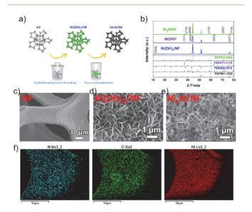
Fig. 1 (a) A schematic of the synthesis process of Ni<sub>3</sub>N; (b) XRD patterns of as-prepared Ni(OH)<sub>2</sub>/NF, NiO/NF and Ni<sub>3</sub>N/NF; (c) SEM image of nickel foam; (d and e) SEM images of as-prepared Ni(OH)2/NF, NiO/NF and Ni<sub>3</sub>N/NF nanosheets; (f) EDX patterns of Ni<sub>3</sub>N/NF.
