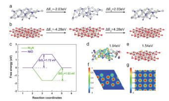
Fig. 4 Schematic slab models of (a)  $Ni_3N$  and (b) NiO. (c) Free energy diagram for the HER on three considered models at zero potential. The charge density difference plots for \*H on (d)  $Ni_3N$  and (e) NiO with an isosurface value of 0.003 e Å<sup>-3</sup>. Yellow and cyan contours represent electron accumulation and depletion of O-intermediate species, respectively. Electron localization function (ELF) for (f)  $Ni_3N$  and (g) NiO.
