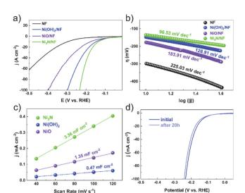
Fig. 3 (a) Polarization curves of Ni $_3$ N, NiO and Ni(OH) $_2$  and Pt/C electrocatalysts. (b) The corresponding Tafel plots of the three catalysts. (c) The  $C_{\rm dl}$  calculations of Ni $_3$ N, NiO and Ni(OH) $_2$ . (d) Polarization curves of Ni $_3$ N/NF in 1 m KOH before and after 20 h under a certain potential (at -0.15 V vs. RHE).
