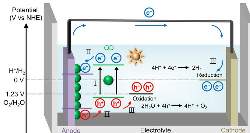
Fig. 1 Schematic illustration depicting the general working principle of QD-based PEC devices.
