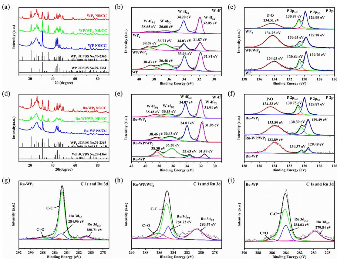
**Fig. 3** (a) XRD patterns of  $WP_2$  and  $WP/WP_2$  WP nanosheet arrays. XPS spectra of (b) W 4f and (c) P 2p of  $WP_2$  and  $WP/WP_2$  WP nanosheet arrays. (d) XRD patterns of Ru- $WP_2$ , Ru- $WP/WP_2$  and Ru-WP nanosheet arrays. XPS spectra of (e) W 4f, (f) P 2p, (g–i) C 1s and Ru 3d of Ru- $WP_2$ , Ru- $WP/WP_2$  and Ru-WP nanosheet arrays.
