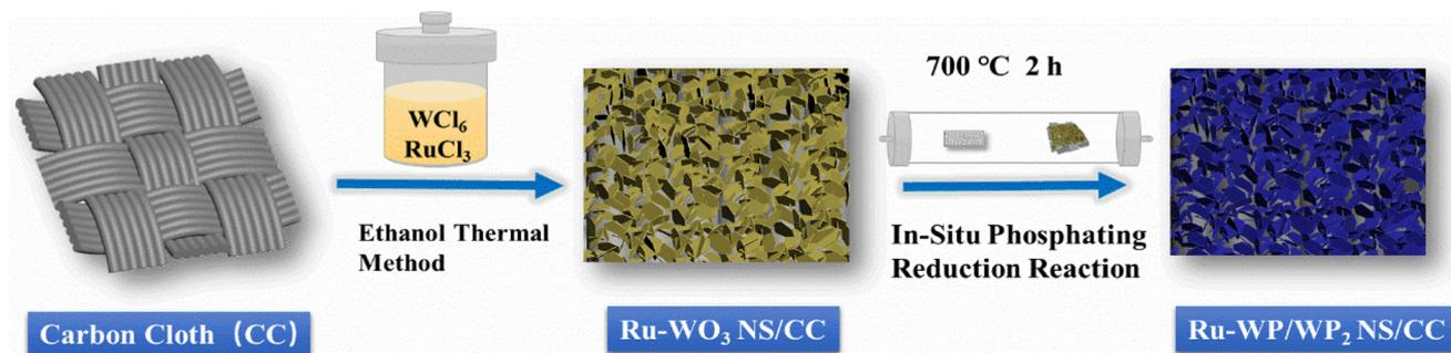
Fig. 1 Schematic illustration of the fabrication of Ru-WP/WP<sub>2</sub> NH/CC.
