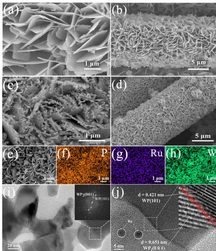
Fig. 2 SEM images of (a and b)  $Ru-WO_3$  NH/CC and (c and d)  $WP/WP_2$  NH/CC samples with different magnifications. (e–h) EDS elemental mapping analysis of P, W, and Ru in the  $Ru-WP/WP_2$  NH/CC sample. (i and j) HR-TEM images of  $Ru-WP/WP_2$  NH/CC.
