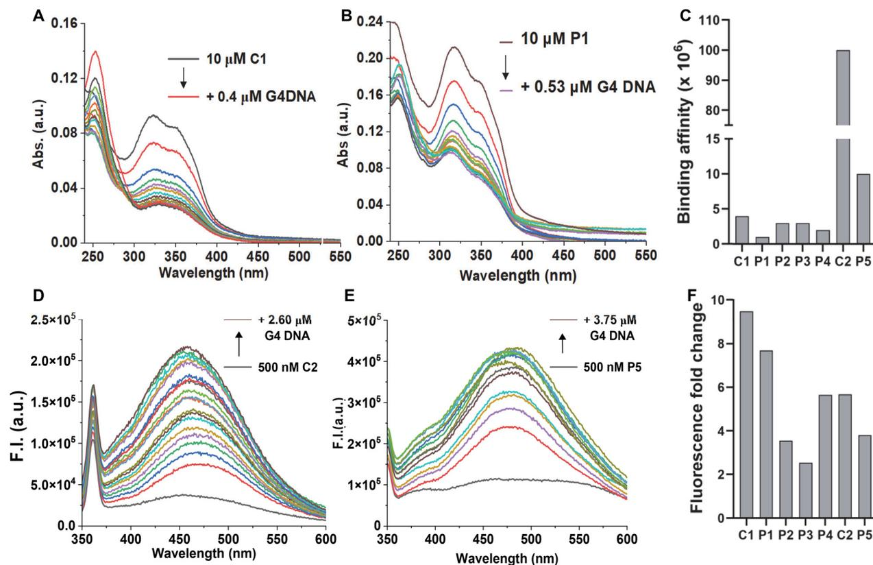
**Fig. 5** UV-Vis titration spectra of 10  $\mu\text{M}$  ligands (A) C1 and (B) P1, and (C) binding affinities for all the molecules in 10 mM Tris-HCl (pH 7.4), 0.1 mM EDTA and 0.1 M KCl with 10  $\mu\text{M}$  pre-formed Hum 21-mer G4 DNA. Fluorescence titration spectra of 0.5  $\mu\text{M}$  ligands (D) C2 and (E) P5, and (F) fold change for all the molecules in 10 mM Tris-HCl (pH 7.4), 0.1 mM EDTA and 0.1 M KCl with 10  $\mu\text{M}$  pre-formed Hum 21-mer G4 DNA.
