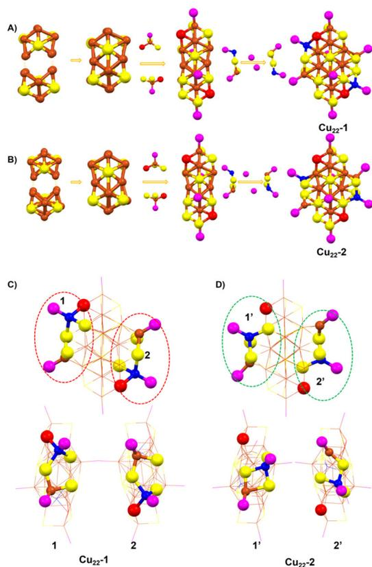
**Fig. 2** (A and B) Anatomy of the two  $\text{Cu}_{22}$  clusters. The copper atoms highlighted in blue and Se atom highlighted in red represent a slight change in bonding patterns in the surface structure. (C and D) The different bonding environments of  $\text{Cu}_2(\text{SeR})_2(\text{PR}_3)_2$  motifs with the  $\text{Cu}_{16}\text{Se}_6@(\text{Cu}_2(\text{SeR})_6(\text{PR}_3)_2)$  framework. Cu = brown/blue, Se = yellow/red, P = purple. For clarity, C, H and F atoms are omitted.
