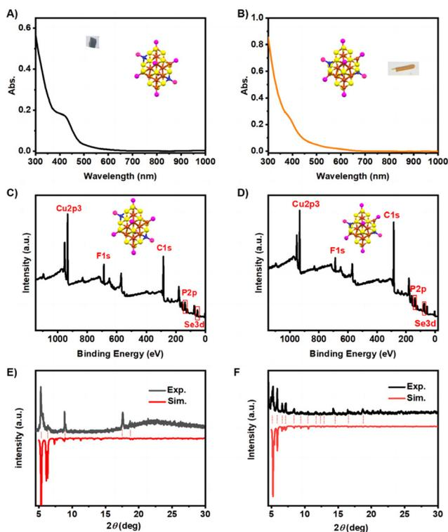
Fig. 4 The UV-vis spectra of isomeric (A)  $\text{Cu}_{22-1}$  dissolved in  $\text{CH}_2\text{Cl}_2$  and (B)  $\text{Cu}_{22-2}$  slightly dissolved in  $\text{CH}_2\text{Cl}_2$ ; the XPS data of (C)  $\text{Cu}_{22-1}$  and (D)  $\text{Cu}_{22-2}$ ; the PXRD data of (E)  $\text{Cu}_{22-1}$  and (F)  $\text{Cu}_{22-2}$ .
