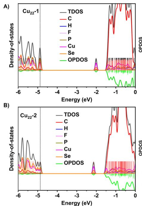
Fig. 5 Calculated PDOS for (A)  $\text{Cu}_{22-1}$  and (B)  $\text{Cu}_{22-2}$ . Here the orbital energy range is set from -6 eV to 0 eV.
