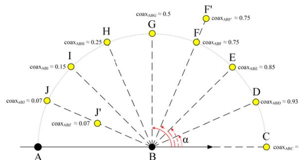
Fig. 7 Illustration of the idea of angular coaxiality, where the last point and last but one point of the line are marked in black and the yellow points are candidates for adding to the line.
