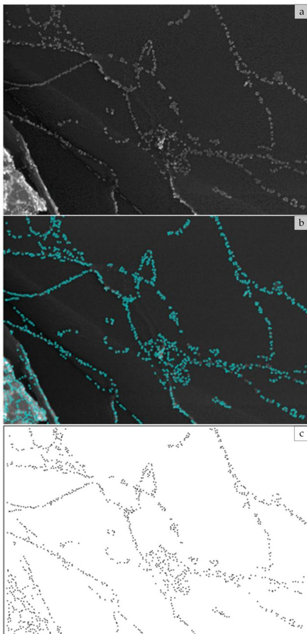
**Fig. 2** Image analysis: (a) the original SEM image; (b) the nanoparticles arrangement in the background of the SEM image; and (c) the map of nanoparticles arrangement used for order analysis.
