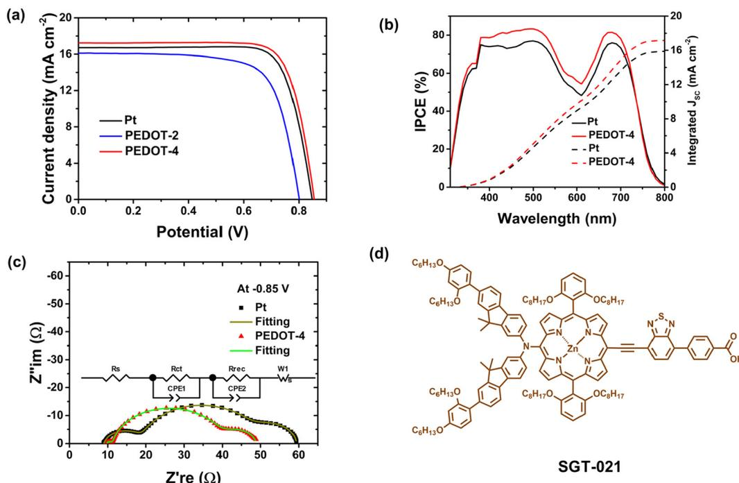
Fig. 7 (a)  $J$ - $V$  curves, (b) IPCE with integrated current density, and (c) Nyquist plots of DSSCs using PEDOT and Pt-counter electrodes. (d) The structure of porphyrin dye used to fabricate the device.
