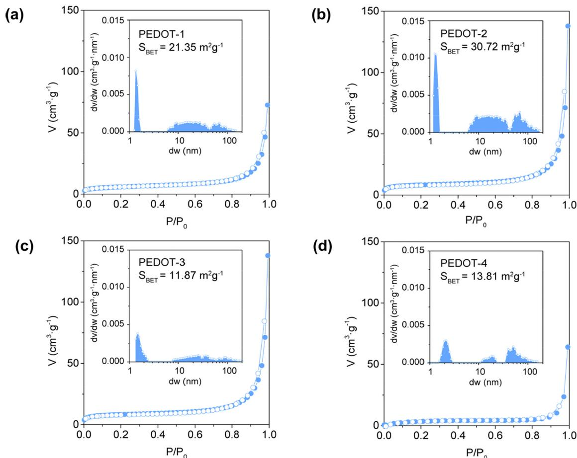
**Fig. 3**  $N_2$  adsorption/desorption isotherms with inset figures representing pore size distribution based on  $N_2$  adsorption branch using NLDFT models for carbon slit-shaped pores of (a) PEDOT-1, (b) PEDOT-2, (c) PEDOT-3, and (d) PEDOT-4.
