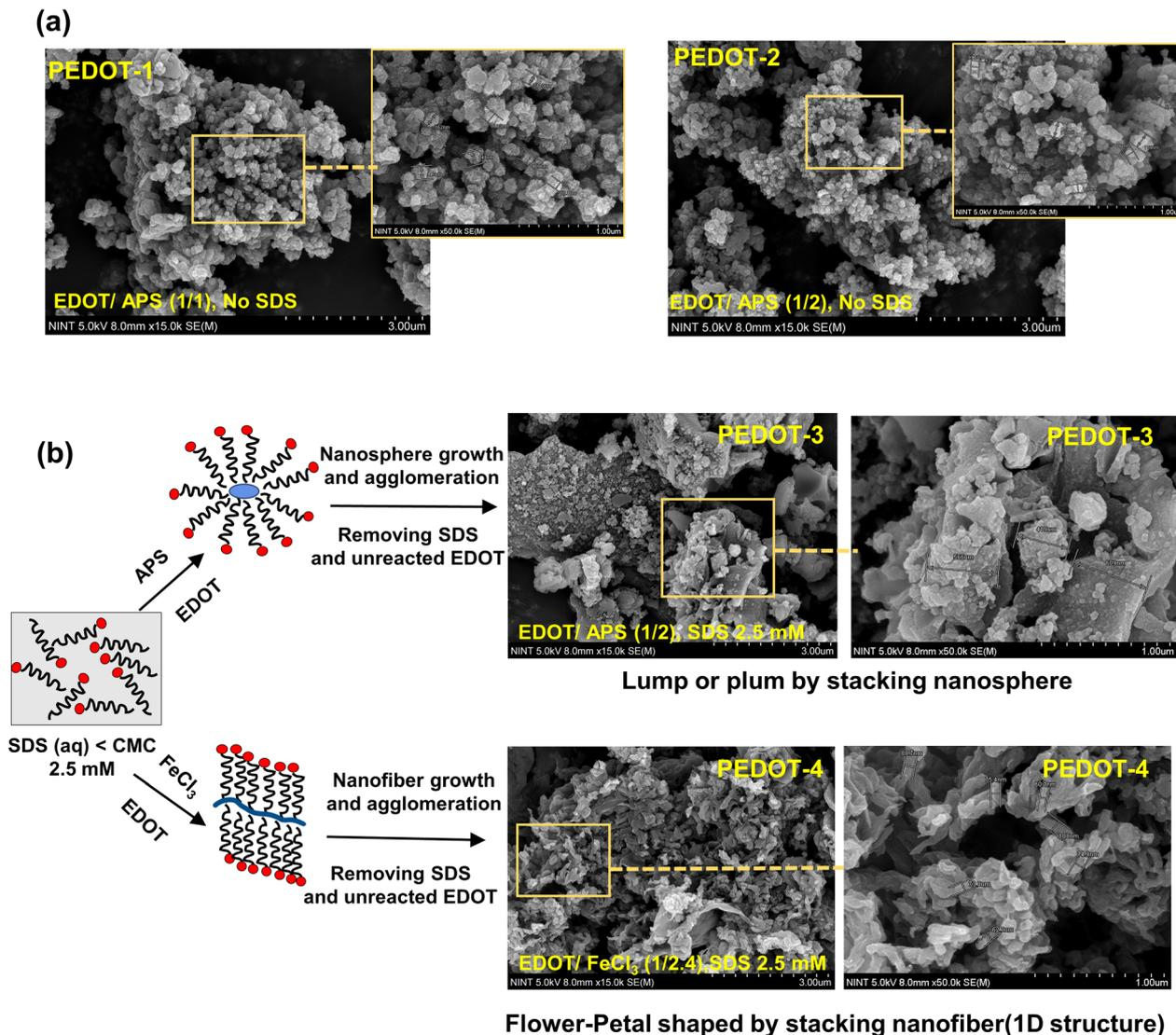
Fig. 2 (a) SEM images of the chemically synthesized PEDOTs using the APS oxidant with varying EDOT to APS concentrations. (b) Morphology of PEDOT-3 and PEDOT-4 synthesized using the APS and  $\text{FeCl}_3$  oxidant, respectively, in the presence of 2.5 mM SDS surfactant.
