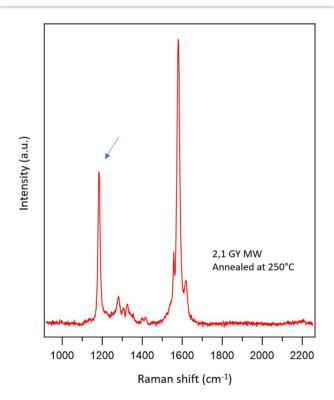
Fig. 7 Experimental Raman spectrum of the 2,1 MWs after annealing at 250 °C.
