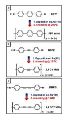
Scheme 1 Representation of the bottom-up growth of different molecular wires on the Au(111) surface: (a) poly-p-phenylene (PPP) wires starting from the 4,4"-dibromo-p-terphenyl (DBTP) precursor; (b) 2,1 graphyne molecular wires (2,1 MWs) from the 1,2-di(4-bromophenyl)-ethyne (DBPE) precursor; (c) 2,2 graphdiyne molecular wires (2,2 MWs) from the 1,4-di(4-bromophenyl)-1,3-butadiyne (DBPB) precursor.
