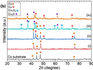
Fig. 2 (a) Energy dispersive X-ray (EDX) spectroscopy profiles and (b) X-ray diffraction patterns of the Co substrate, (i) Co TF, (ii) Co TF + 0.1 M CuSO<sub>4</sub>, (iii) Co/Cu-A, and (iv) Co/Cu-AA catalysts.
