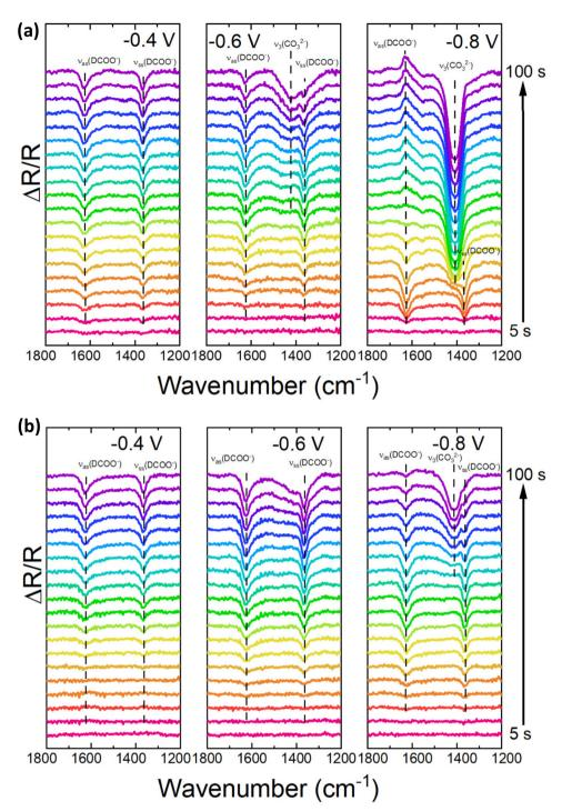
Fig. 6 Time-dependent FTIR spectra in the range of  $1800-1200 \text{ cm}^{-1}$  were recorded during the  $CO_2RR$  using (a) Co/Cu-A and (b) Co/Cu-AA catalysts in a  $CO_2$ -saturated 0.5 M  $K_2SO_4$  solution in  $D_2O$  at -0.4, -0.6, and -0.8 V vs. RHE.
