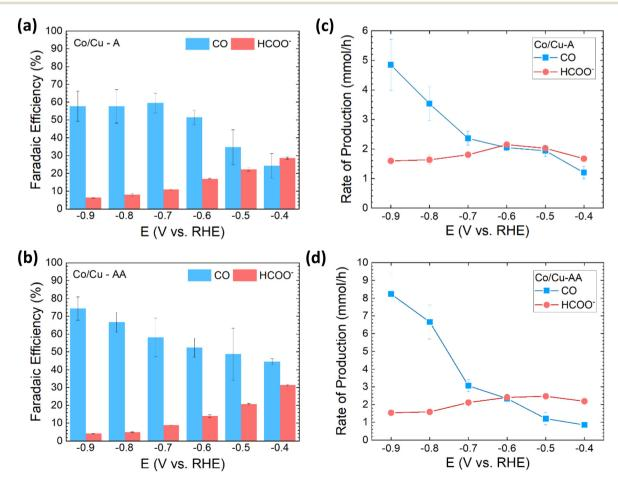
Fig. 4 (a & b) Calculated faradaic Efficiencies of carbon monoxide (CO) and formate ion (HCOO<sup>-</sup>) obtained after 60 min of the applied potential using (a) Co/Cu-A and (b) Co/Cu-AA catalysts. (c & d) Measured CO and HCOO<sup>-</sup> production rates during the CO<sub>2</sub>RR at each applied potential using (c) Co/Cu-A and (d) Co/Cu-AA catalysts.
