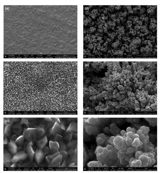
Fig. 1 Scanning electron microscopy (SEM) images of Co/Cu-A (a-c) and Co/Cu-AA (d-f) at 1000x (a and d), 10 000x (b and e), and 100 000x (c and f) magnifications.
