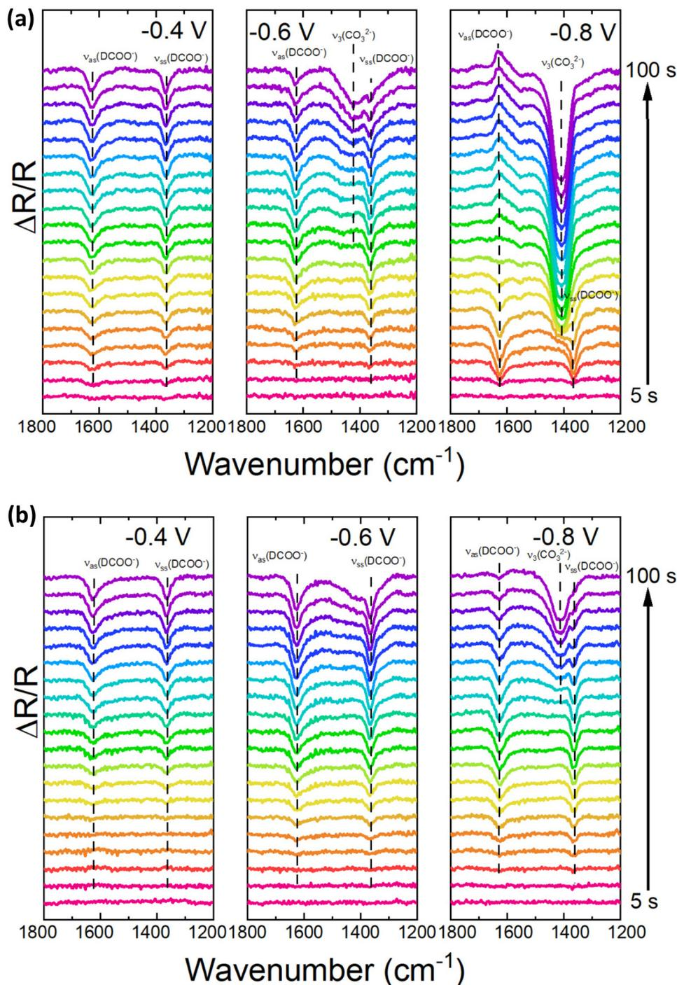
**Fig. 6** Time-dependent FTIR spectra in the range of 1800–1200  $\text{cm}^{-1}$  were recorded during the  $\text{CO}_2\text{RR}$  using (a) Co/Cu–A and (b) Co/Cu–AA catalysts in a  $\text{CO}_2$ -saturated 0.5 M  $\text{K}_2\text{SO}_4$  solution in  $\text{D}_2\text{O}$  at  $-0.4$ ,  $-0.6$ , and  $-0.8$  V vs. RHE.
