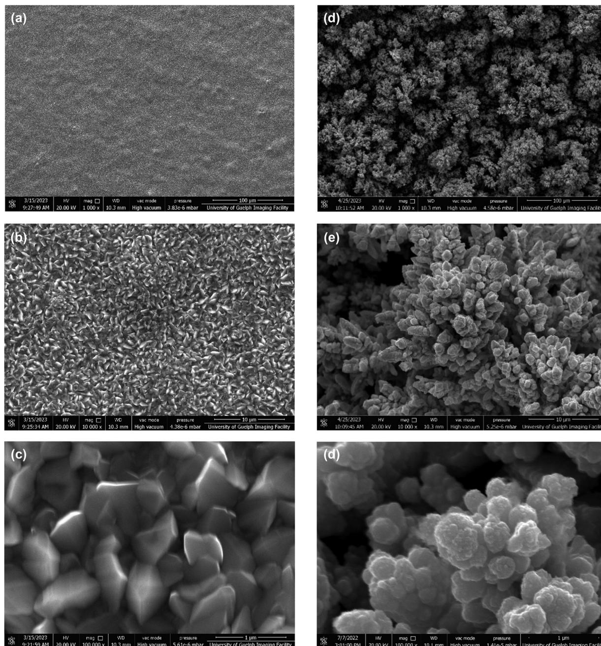
**Fig. 1** Scanning electron microscopy (SEM) images of Co/Cu-A (a–c) and Co/Cu-AA (d–f) at 1000 $\times$  (a and d), 10 000 $\times$  (b and e), and 100 000 $\times$  (c and f) magnifications.
