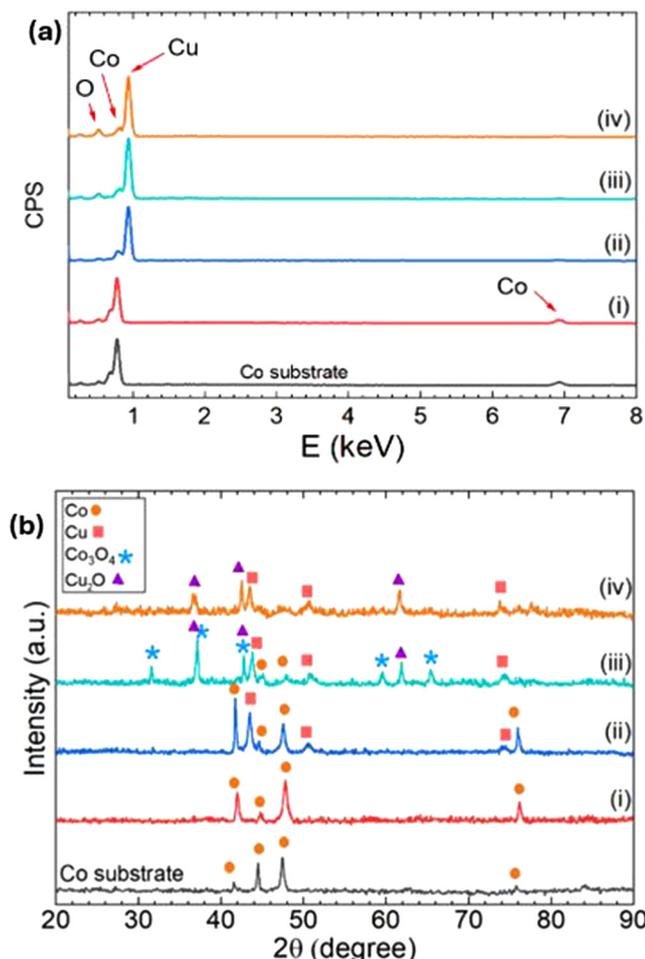
Fig. 2 (a) Energy dispersive X-ray (EDX) spectroscopy profiles and (b) X-ray diffraction patterns of the Co substrate, (i) Co TF, (ii) Co TF + 0.1 M CuSO<sub>4</sub>, (iii) Co/Cu-A, and (iv) Co/Cu-AA catalysts.
