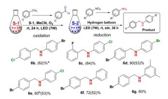
**Fig. 14** One-pot mechanism for assisted tandem catalysis of S-2 and S-1 states to give *N*-benzylaniline derivatives with different substituent groups attached. "Reproduced from ref. 93 with permission from the American Chemical Society, copyright 2018".
