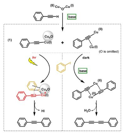
Fig. 10 Sonogashira and Glaser coupling reaction pathways over the Cu<sub>x</sub>O/CNT catalyst under light irradiation and dark conditions respectively. "Reproduced from ref. 89 with permission from Elsevier, copyright 2022".
