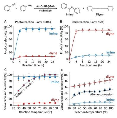
Fig. 17 Hydroamination reaction and homo diyne formation with alkyne and aniline. (A) Reactions carried out with  $Au_2Co/ZrO_2$  under visible light irradiation and (B) in the dark. (C) The effect of temperature under visible light and (D) in the dark. "Reproduced from ref. 107 with permission from John Wiley and Sons, copyright 2019".
