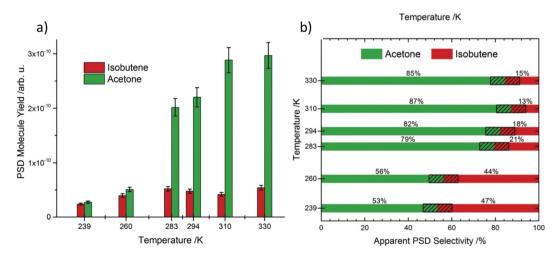
Fig. 3 (a) Integrated molecule yields indicating a higher overall yield at higher temperatures. (b) Selectivity of the products obtained at different temperatures. "Reproduced from ref. 65 with permission from Royal Society of Chemistry, copyright 2018".
