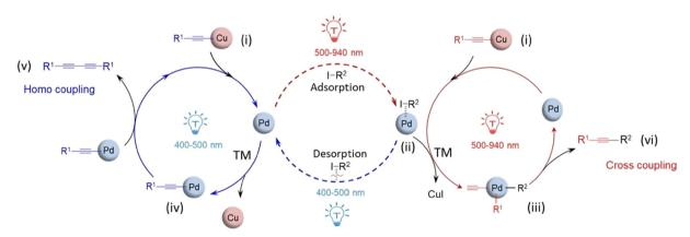
Fig. 12 Proposed mechanism of the coupling reaction with Cu/Pd mixed NPs. Blue circle depicts the mechanism under short-wavelength irradiation and red circle, under long-wavelength irradiation. "Reproduced from ref. 90 with permission from John Wiley and Sons, copyright 2022".
