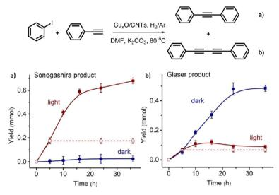
Fig. 9 Yield vs. time graphs of (a) Sonogashira and (b) Glaser reactions under visible light irradiation and dark conditions. 1.0 mmol phenylacetylene, 1.5 mmol iodobenzene, 1.5 mmol K<sub>2</sub>CO<sub>3</sub>, 2 mL DMF, 100 mg Cu<sub>x</sub>O/CNTs, 0.75 W cm<sup>-2</sup>, 80 °C, H<sub>2</sub>/Ar. "Reproduced from ref. 89 with permission from Elsevier, copyright 2022".
