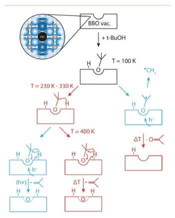
Fig. 2 Reaction mechanism that occurs on the r-TiO<sub>2</sub>(110) surface. Photochemical pathways are indicated in blue and thermocatalytic steps in red. "Reproduced from ref. 65 with permission from the Royal Society of Chemistry, copyright 2018".
