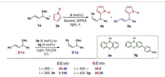
Fig. 20 Photocatalytic allylation reaction and Isomerization studies of *E-1a* with photocatalysts 3e and 3g under different irradiation wavelengths. "Reproduced from ref. 115 with permission from Springer Nature, copyright 2019".
