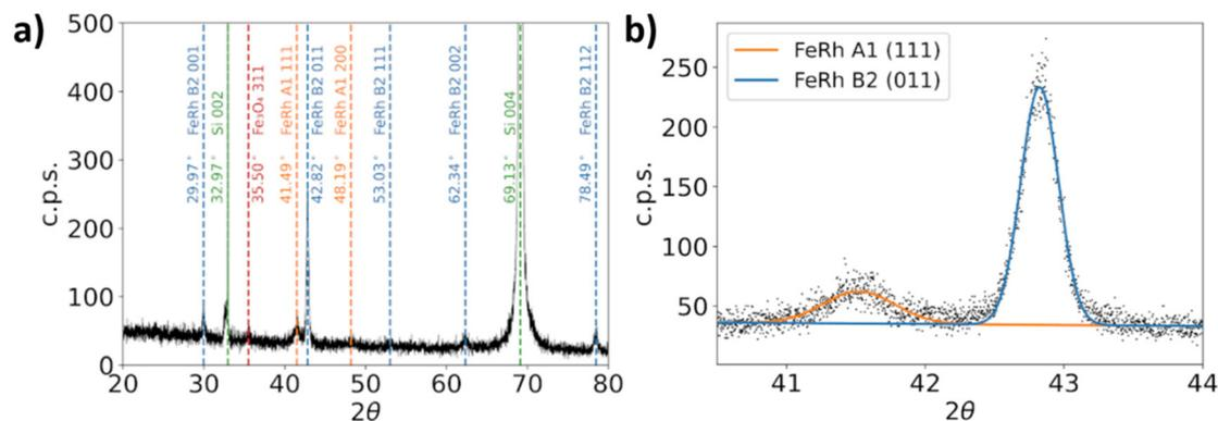
**Fig. 2** Specular XRD pattern of the FeRh nanocluster assembled film with labelled peak positions of FeRh A1 phase (orange), FeRh B2 phase (blue), Si (green) and Fe<sub>3</sub>O<sub>4</sub> (red) (a). Magnification of the XRD pattern in the region of FeRh A1 (111) and FeRh B2 (011) peaks with Gaussian fits using the Scherrer formula with shape factor 0.9 (b).
