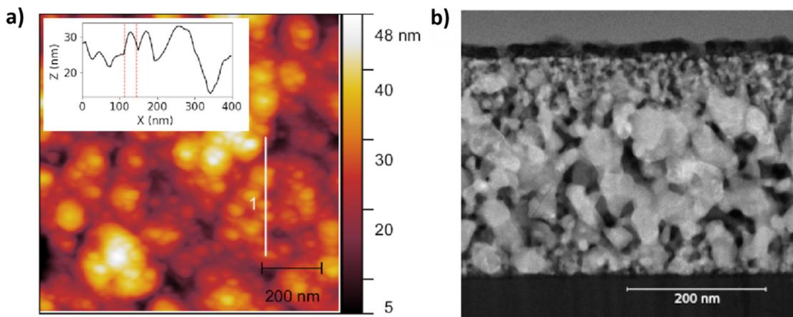
**Fig. 1** AFM top view of the FeRh nanocluster assembled film with 150 nm nominal thickness measured in tapping mode (a), and topography profile along line 1 (white) with a 30 nm length dome delimited with the red vertical dotted lines (inset). STEM-HAADF lateral view on a cross-section lamella of the FeRh nanocluster assembled film (b).
