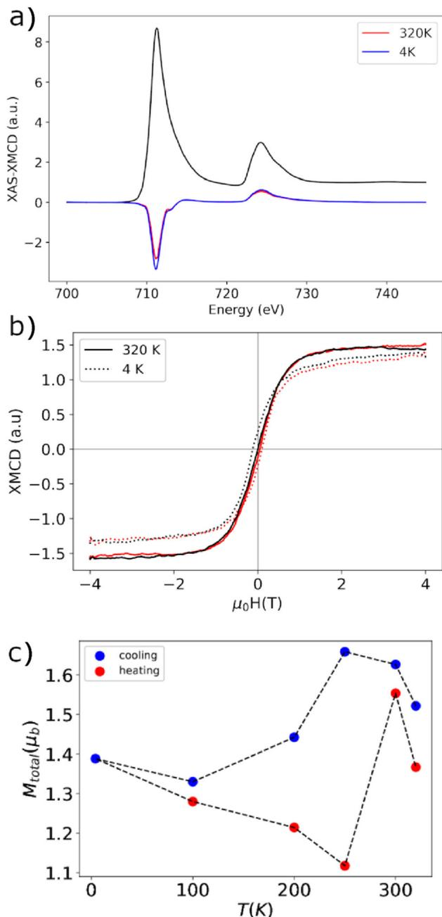
**Fig. 6** XAS and XMCD in the soft X-ray regime measured on the annealed FeRh nanocluster assembled film at the Fe L-edge in TEY mode under 6 T and perpendicular incidence leading to a total magnetic moment of  $1.4\mu_B$  at 4 K and  $1.5\mu_B$  at 320 K (a). XMCD signal taken as the max XAS value at the Fe  $L_3$  edge versus the applied magnetic field (b). Temperature dependence of the Fe total magnetic moment measured from the thermal XMCD evolution under 6 T (c).
