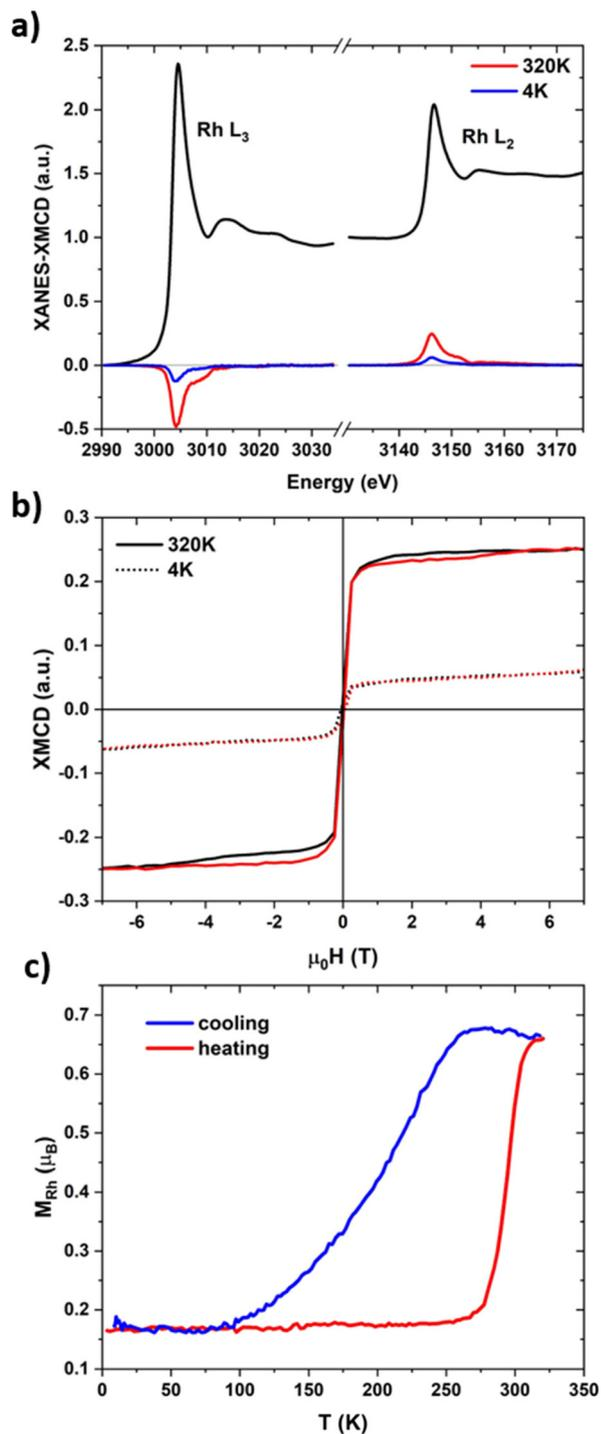
Fig. 5 XAS and XMCD in the hard X-ray regime measured on the annealed FeRh nanocluster assembled film in TFY mode at the Rh L<sub>2</sub>-edge under 7 T and 15° grazing incidence leading to a total magnetic moment of 0.16 μ<sub>B</sub> at 4 K and 0.65 μ<sub>B</sub> at 320 K (a). XMCD signal taken as the maximum XAS value at the L<sub>2</sub>-edge versus the applied magnetic field (b). Temperature dependence of the Rh total magnetic moment measured from thermal XMCD evolution under 7 T (c).
