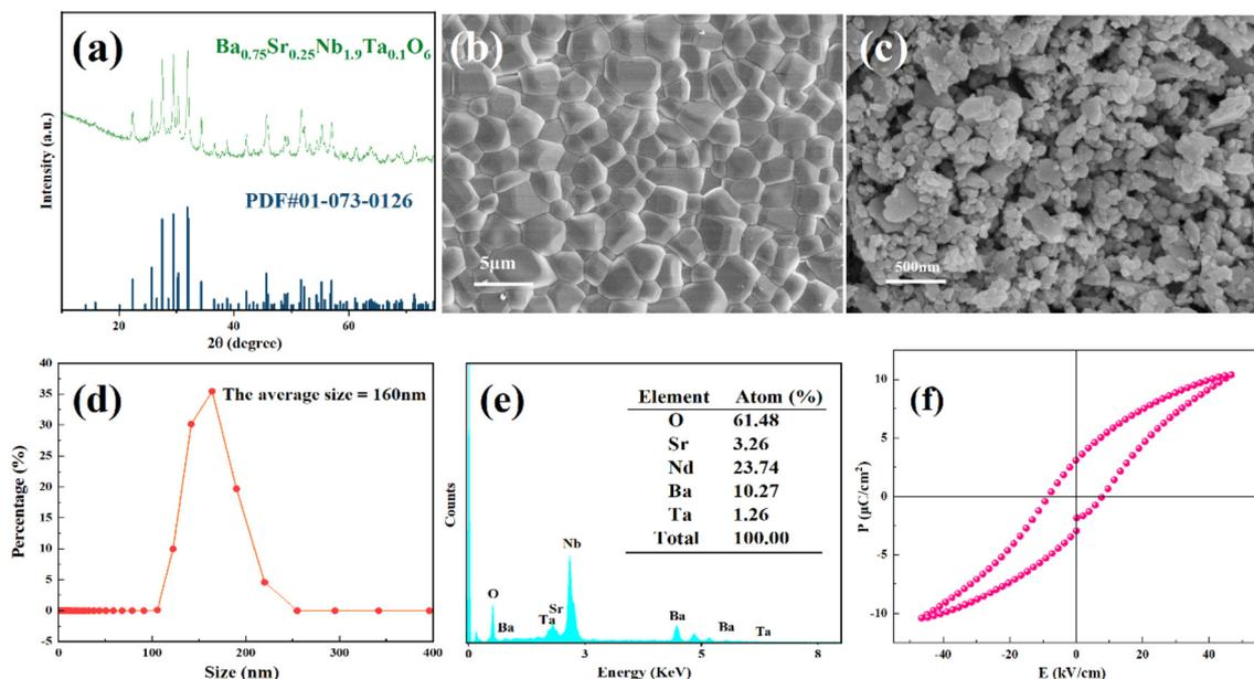
**Fig. 1** (a) XRD diffraction pattern of the BSNT powder after high-energy ball milling, (b) SEM image of the BSNT ceramic, (c) SEM image of the BSNT powder after high-energy ball milling, (d) particle size distribution after high-energy ball milling, (e) EDS energy spectrum of BSNT, and (f)  $P$ - $E$  loop of the BSNT ceramic measured at 700 V and 10 Hz at room temperature.
