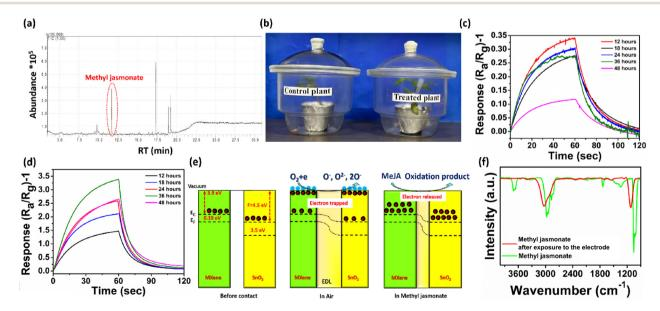
Fig. 5 (a) GC-MS chromatogram obtained from the head-space volatiles of the tomato plant infested with Tuta-absoluta. (b) Photographs of the incubated control and treated plants. Sensor response to the (c) control plant and (d) treated plant at different time periods. (e) Energy diagram of the SnO<sub>2</sub>/MXene nanocomposite. (f) FTIR spectra of MeJA before and after exposure to the electrode.
