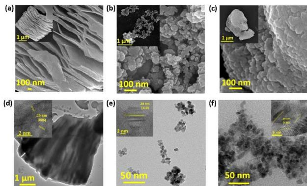
Fig. 2 Scanning electron microscopy images of the (a) MXene, (b) SnO<sub>2</sub> and (c) SnO<sub>2</sub>/MXene nanocomposite. Transmission electron microscopy images of (d) MXene, (e) SnO<sub>2</sub> and (f) SnO<sub>2</sub>/MXene.
