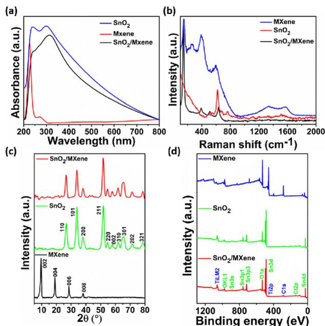
**Fig. 1** Characterization of the SnO<sub>2</sub>, MXene and SnO<sub>2</sub>/MXene nanocomposite. (a) UV-Vis spectra, (b) Raman spectra, (c) XRD spectra and (d) XPS survey spectra of the SnO<sub>2</sub>, MXene and SnO<sub>2</sub>/MXene nanocomposite.
