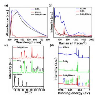
Fig. 1 Characterization of the SnO<sub>2</sub>, MXene and SnO<sub>2</sub>/MXene nanocomposite. (a) UV-Vis spectra, (b) Raman spectra, (c) XRD spectra and (d) XPS survey spectra of the SnO2, MXene and SnO2/MXene nanocomposite.
