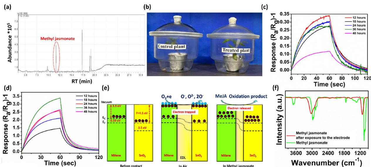
**Fig. 5** (a) GC-MS chromatogram obtained from the head-space volatiles of the tomato plant infested with *Tuta-absoluta*. (b) Photographs of the incubated control and treated plants. Sensor response to the (c) control plant and (d) treated plant at different time periods. (e) Energy diagram of the SnO<sub>2</sub>/MXene nanocomposite. (f) FTIR spectra of MeJA before and after exposure to the electrode.
