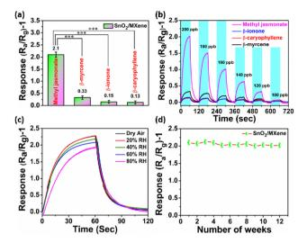
Fig. 4 (a and b) Selectivity of the SnO<sub>2</sub>/MXene sensor for MeJA against different analytes with a concentration gradient. The stability of the sensor (c) under different RHs (d) for continuous 12 weeks. Three independent experiments were conducted, and the response obtained with methyl jasmonate was compared with those of  $\beta$ -ionone,  $\beta$ -caryophyllene, and  $\beta$ -myrcene. Results are given as mean  $\pm$  SD. Statistical significance is shown by \*\*\* $p \le 0.001$ .
