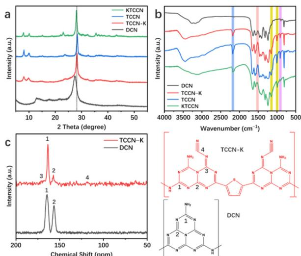
**Fig. 2** XRD patterns (a) and FT-IR spectra (b) of DCN, TCCN-K, TCCN and KTCCN; (c) solid-state <sup>13</sup>C MAS NMR spectra and the corresponding structure of TCCN-K and DCN.
