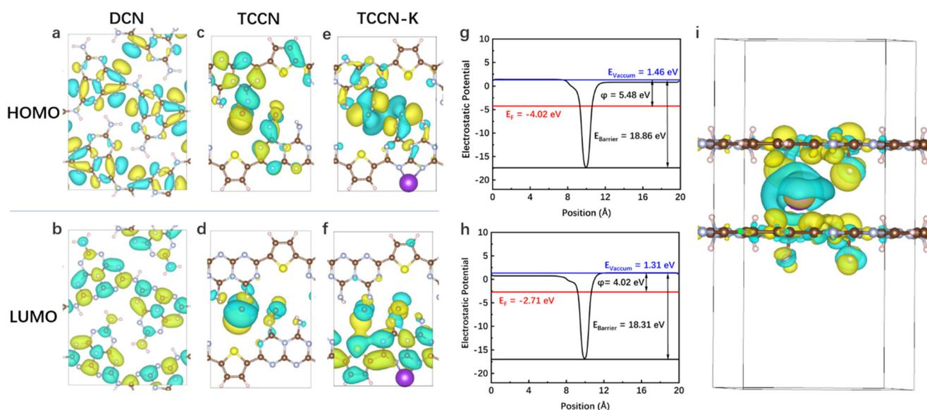
**Fig. 7** HOMO and LUMO distribution of DCN (a and b), TCCN (c and d) and TCCN-K (e and f); calculated work function and layered electrostatic potential energy of TCCN (g) and TCCN-K (h); and charge density difference of TCCN-K (i).
