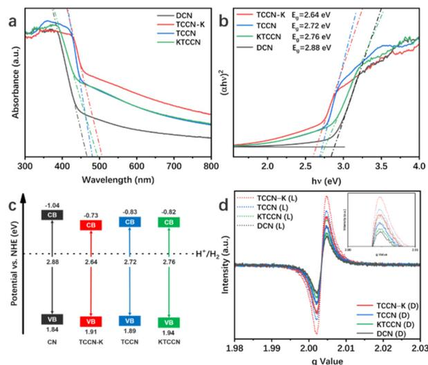
**Fig. 4** UV-vis spectra (a), the corresponding Tauc plots derived from the Kubelka–Munk rule (b) and experimental energy band structure diagram (c) of all samples; (d) EPR spectra of DCN, TCCN and TCCN-K under dark (D) and light (L) conditions.
