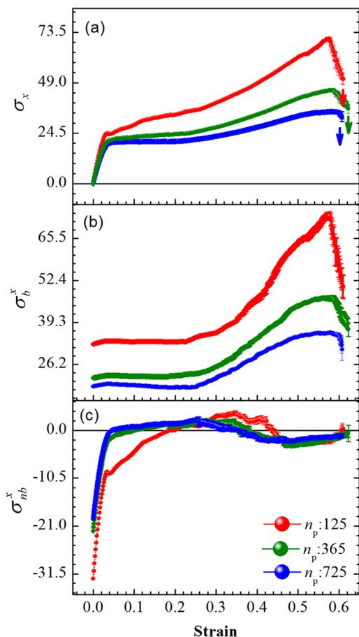
**Fig. 4** Average forces per unit thickness,  $\sigma = F/W$ , on the right edge of the PGP array along the direction of stretching as a function of strain at constant pulling velocity,  $u = 0.001u_0$ , and  $E = 39k_B T$ . (a) The net force,  $\sigma_x: F_x/W$ , (b) bonded contributions,  $\sigma_b^x: F_b/W$  and (c) non-bonded contributions,  $\sigma_{nb}^x: (F_{nb}^{rep} + F_{nb}^{coh})/W$ .
