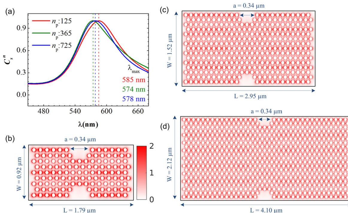
**Fig. 2** (a) Normalized scattering cross section,  $C_s^n$ , as a function of wavelength for three PGPN arrays composed of 125 (red curve), 365 (green curve) and 725 (blue curve) PGPNs. Electric field amplitude on the  $xy$ -plane (where  $z = 0$ ) for the arrays with (b) 125, (c) 365 and (d) 725 PGPNs. The structure is illuminated with an  $X$ -polarized plane wave propagating in the  $z$  direction. The electric field maps are calculated at the resonance wavelengths,  $\lambda_{\max}$ .
