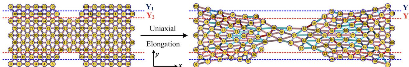
**Fig. 3** Schematic of the uniaxial elongation of the PGPN array at a constant pulling velocity  $u = 0.001u_0$  in the  $x$  direction. The snapshot of the deformed array is provided at an elongational strain of  $\alpha = 0.6$ . The horizontal dashed blue and red lines demarcate the regions  $Y_1$  and  $Y_2$ , which are normal to the direction of elongation ( $y$  direction), respectively. The number of PGPNs within the demarcated regions evolves with strain.
