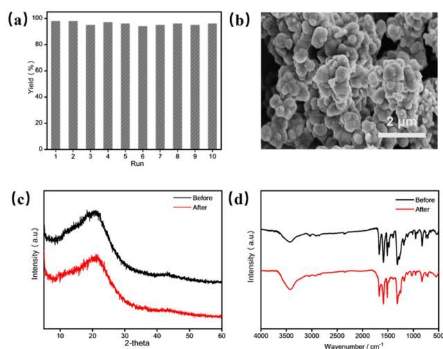
**Fig. 4** (a) Reusability of PAF-380 in the photocatalytic synthesis of benzimidazole of **1a** and **2a**. (b) SEM image of PAF-380 after ten cycles. (c) PXRD patterns of PAF-380 before and after ten cycles. (d) FTIR spectra of PAF-380 before and after ten cycles.
