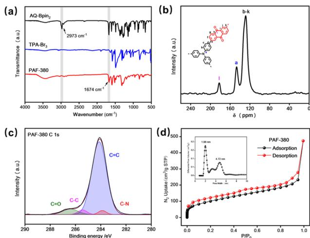
**Fig. 1** (a) FTIR spectra of PAF-380 and starting materials. (b) The solid-state  $^{13}\text{C}$  CP/MAS NMR spectrum of PAF-380. (c) XPS C 1s spectrum of PAF-380. (d) Nitrogen adsorption–desorption isotherm at 77 K and the corresponding pore size distribution profile.
