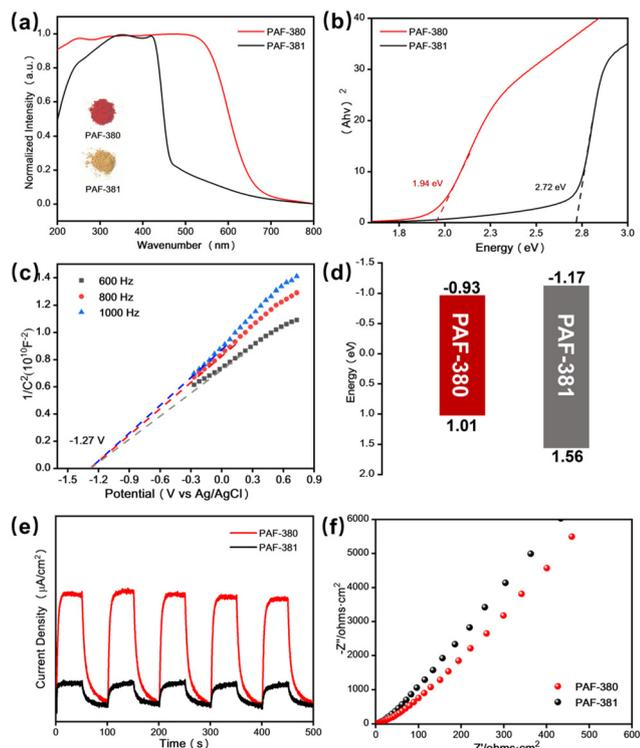
**Fig. 3** (a) Solid-state absorption profiles of TPA-PAFs, insets: the corresponding images. (b) Tauc plots of TPA-PAFs. (c) Mott-Schottky plots of PAF-380. (d) Schematic energy band structure of TPA-PAFs. (e) Transient photocurrent response graph of TPA-PAFs under light irradiation. (f) The Nyquist plots of TPA-PAFs.
