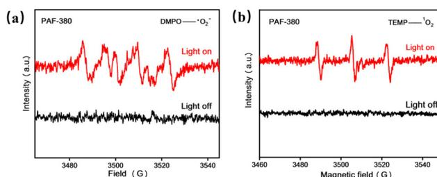
**Fig. 5** (a) ESR spectra of PAF-380 (2.0 mg mL<sup>-1</sup>) and DMPO (0.1 M) in methanol under ambient atmosphere under light irradiation (top) and in darkness (bottom). (b) ESR spectra of PAF-380 (2.0 mg mL<sup>-1</sup>) and TEMP (0.1 M) in methanol under ambient atmosphere under light irradiation (top) and in darkness (bottom).
