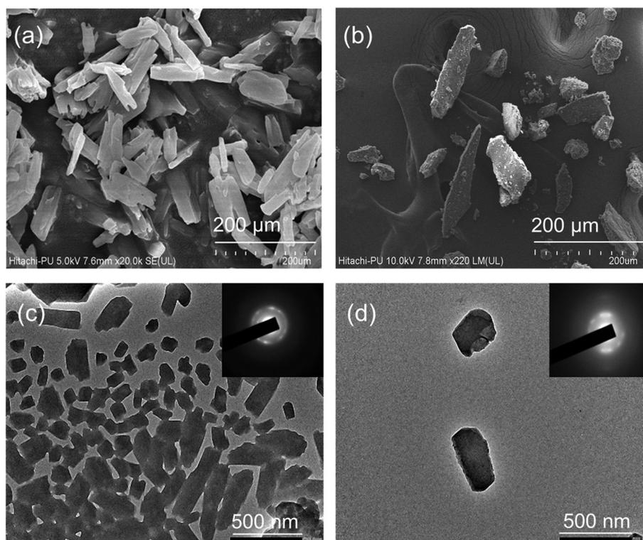
**Fig. 1** Morphological characterization studies. (a) SEM image of Bio-MOF-1; (b) SEM image of Bio-MOF-1/AA; (c) TEM image and the SAED pattern of Bio-MOF-1; and (d) TEM image and the SAED pattern of Bio-MOF-1/AA.
