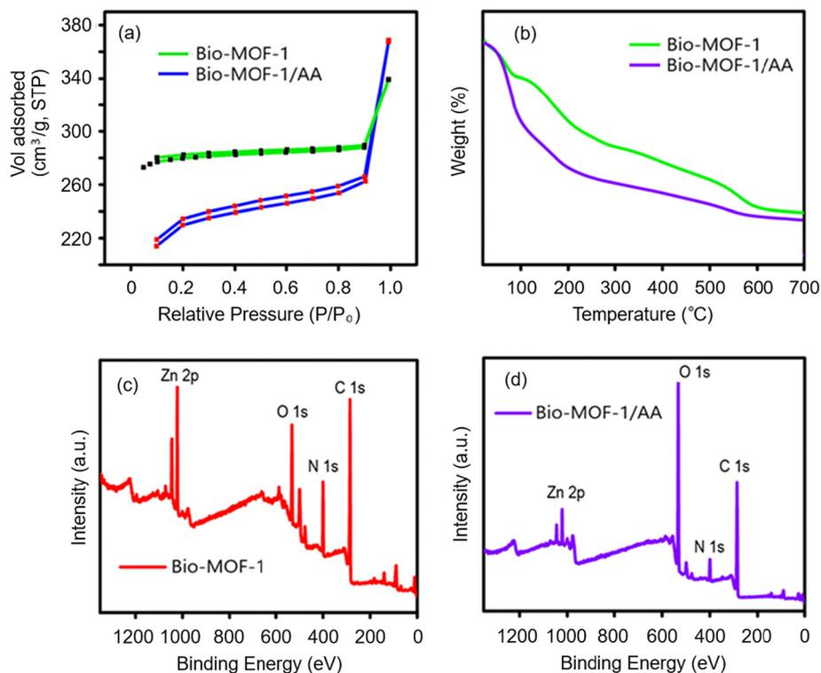
**Fig. 3** Material characterization studies of the synthesized products. (a) BET surface analysis of Bio-MOF-1/AA; (b) TGA curve of Bio-MOF-1/AA; and (c and d) XPS spectra of Bio-MOF-1 and Bio-MOF-1/AA.
