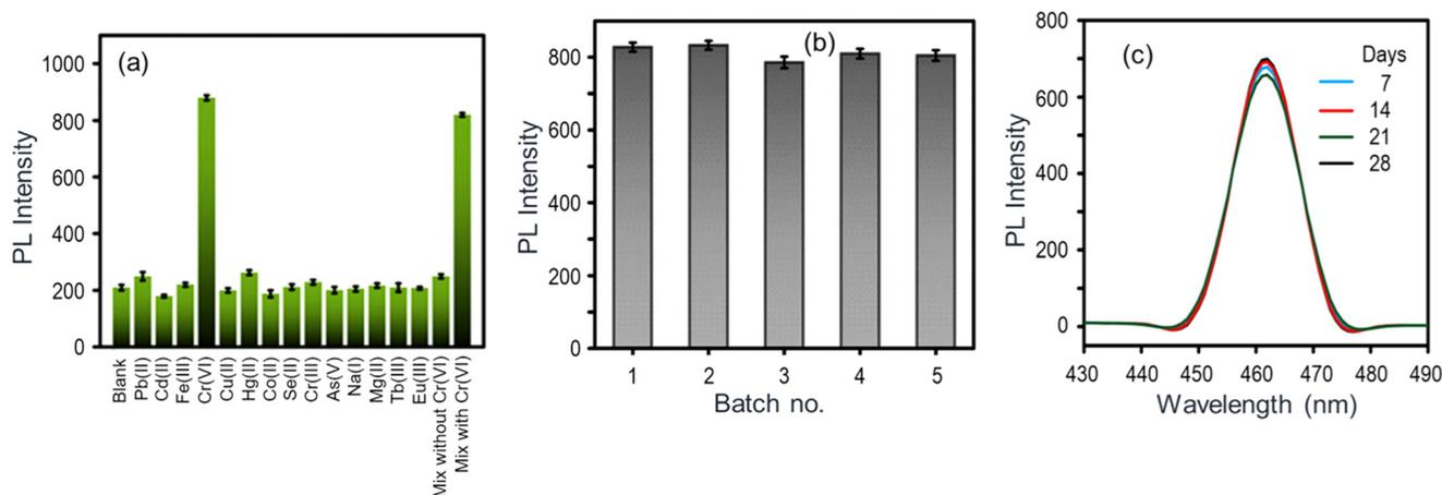
**Fig. 6** Assessment of different important quality assurance aspects of the Bio-MOF-1/AA nanoprobe. (a) Sensor response in terms of PL enhancement toward Cr(vi) and various other potentially co-existing metal ions; (b) PL response of five different nanoprobe solutions against  $10 \text{ ng mL}^{-1}$  Cr(vi); and (c) PL spectra of the nanoprobe solution stored for 4 weeks.
