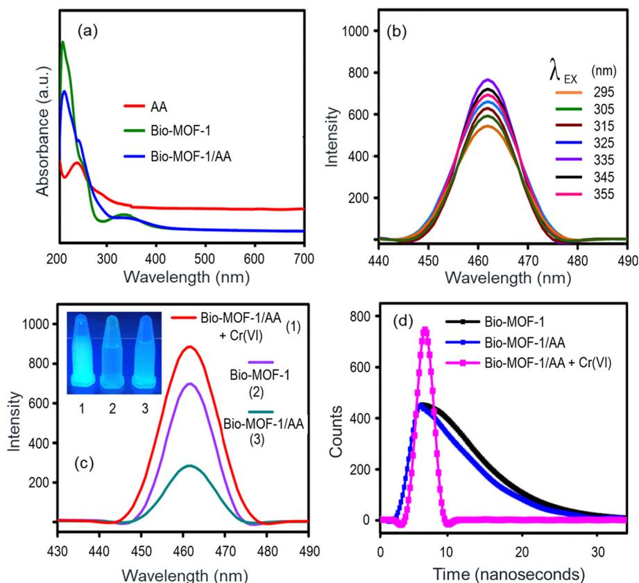
**Fig. 4** Spectrophotometric properties. (a) UV-Vis spectra of Bio-MOF-1, AA, and Bio-MOF-1/AA; (b) PL spectra of Bio-MOF-1 at different excitation wavelengths; (c) PL spectra of Bio-MOF-1, Bio-MOF-1/AA, and Bio-MOF-1/AA-Cr(vi) samples; the inset shows the photograph of samples under a UV trans-illuminator; and (d) fluorescence decay curves of Bio-MOF-1, Bio-MOF-1/AA, and Bio-MOF-1/AA-Cr(vi) samples.
