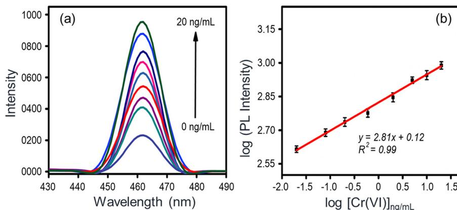
**Fig. 5** Detection of Cr(vi) with the Bio-MOF-1/AA nanoprobe. (a) PL spectra in the presence of varying analyte concentrations (0.02, 0.08, 0.2, 0.6, 2, 5, 10, and 20 ng mL<sup>-1</sup>) and (b) calibration plot between the PL intensity and Cr(vi) concentrations. Experimental conditions: pH = 7.0, [Bio-MOF-1/AA] = 2 mg mL<sup>-1</sup>, excitation wavelength = 335 nm; error bars are based on standard deviations observed in triplicate analysis.
