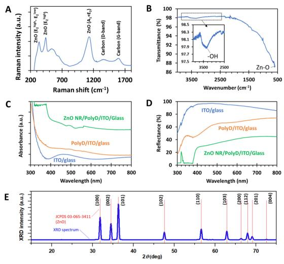
Fig. 3 (A) Raman spectroscopy spectrum of ZnO nanorods (ZnO-nr) on carbon cloth (CC). (B) FTIR spectroscopy spectrum of ZnO nanorods (ZnOnr) on ITO/glass. (C) Optical absorbance and (D) reflectance of ZnO nanorods (ZnO-nr) on ITO/glass samples at various stages of material synthesis. (E) X-ray diffraction spectrum of ZnO nanorods on carbon cloth.
