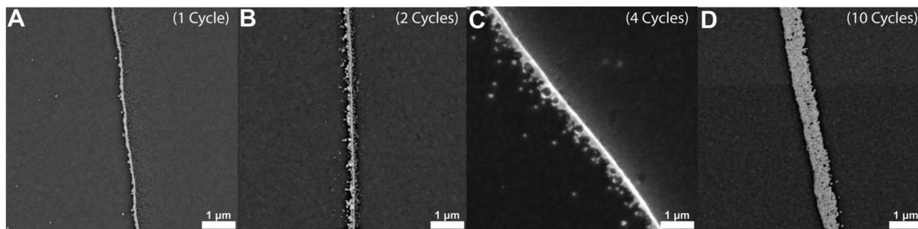
Fig. 3 Scanning electron microscopy images of electrodeposited nanowires of varying widths. A multipotential step chronoamperometric method of biasing the ITO electrode at  $-0.65$  V vs. Ag|AgCl for 0.5 s, followed by 0.3 V vs. Ag|AgCl for 0.5 s was repeated for (A) 1 cycle, (B) 2 cycles, (C) 4 cycles, and (D) 10 cycles.
