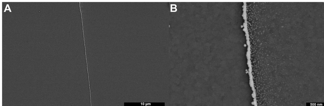
Fig. 2 Scanning electron microscopy (SEM) images taken after 1 cycle of 0.5 s at  $-0.65$  V vs. Ag|AgCl, then 0.5 s at 0.3 V vs. Ag|AgCl for a two-phase system. Images (A) through (B) show increasing magnifications of the same electrode.
