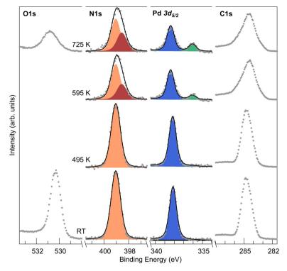
Fig. 4 XPS measurements of a monolayer PdTPP/CuO. Evolution of N 1s, Pd 3d<sub>5/2</sub> and C 1s measured at room temperature after annealing at the indicated T values
