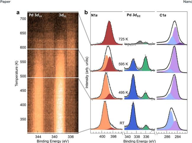
Fig. 1 Evolution of a monolayer of PdTPP/Cu(100) as a function of temperature: (a) temperature-dependent Pd 3d core level spectra upon linear annealing; (b) N 1s, Pd 3d<sub>5/2</sub> and C 1s core levels collected at RT after stepwise annealing to the indicated temperature values (corresponding cutlines in (a) are shown for best clarity).
