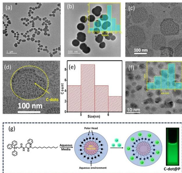
**Fig. 3** (a) Cryo-TEM and (b) FEG-TEM images of the P (inset, size-distribution plot). (c) FEG-TEM images of the CDTP and the zoomed-in version (d). (e) Size-distribution plot of the C-dots and CDTP (f) FEG-TEM images of the C-dots and size-distribution plot (inset). (g) Graphical presentation of the P in water and in the CDTP.
