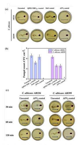
Fig. 6 Antifungal activity of coated surfaces against the drug-resistant fungi C. albicans AB226 and C. albicans AB399 determined (a) through the dragging method, (b) reduction in fungal count and (c) fungicidal kinetics of uncoated and APN3 coated surfaces; arrows indicate the direction of dragging of surfaces on YPD agar plates. An asterisk (\*) indicates a fungal count of <50 CFU per cm<sup>2</sup>.
