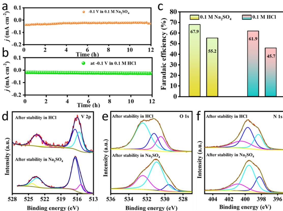
**Fig. 6** (a and b) CA response of VO<sub>2</sub>@CN during the NRR at -0.1 V vs. RHE in 0.1 M Na<sub>2</sub>SO<sub>4</sub> and 0.1 M HCl, respectively, for a continuous 12 h period; (c) FE comparison of the catalyst after 1 and 12 h of NRR studies in both electrolytes; post-NRR XPS profiles for (d) V 2p, (e) O 1s and (f) N 1s, respectively, under HCl and Na<sub>2</sub>SO<sub>4</sub> electrolyte conditions.
