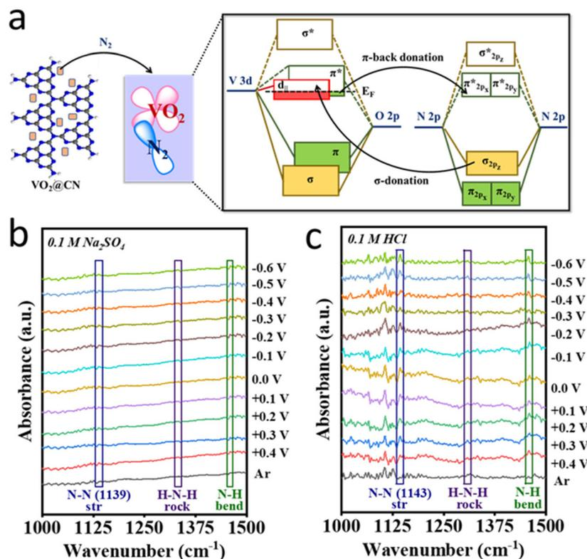
Fig. 5 (a) Orbital interaction between the  $\text{VO}_2$  part of  $\text{VO}_2@\text{CN}$  and  $\text{N}_2$  in terms of a molecular orbital diagram; unprocessed *in situ* ATR-FTIR spectra of the catalyst at different working potentials under  $\text{N}_2$ - and Ar-purged conditions in (b) 0.1 M  $\text{Na}_2\text{SO}_4$  and (c) 0.1 M  $\text{HCl}$ , respectively.
