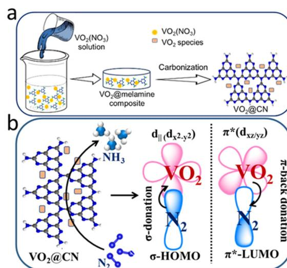
**Fig. 1** (a) Schematic representation of the synthesis of  $\text{VO}_2@\text{CN}$ ; (b) orbital interaction between  $\text{N}_2$  and the  $\text{VO}_2$  centre of the catalyst, responsible for  $\text{N}_2$  reduction to  $\text{NH}_3$  (NRR).
