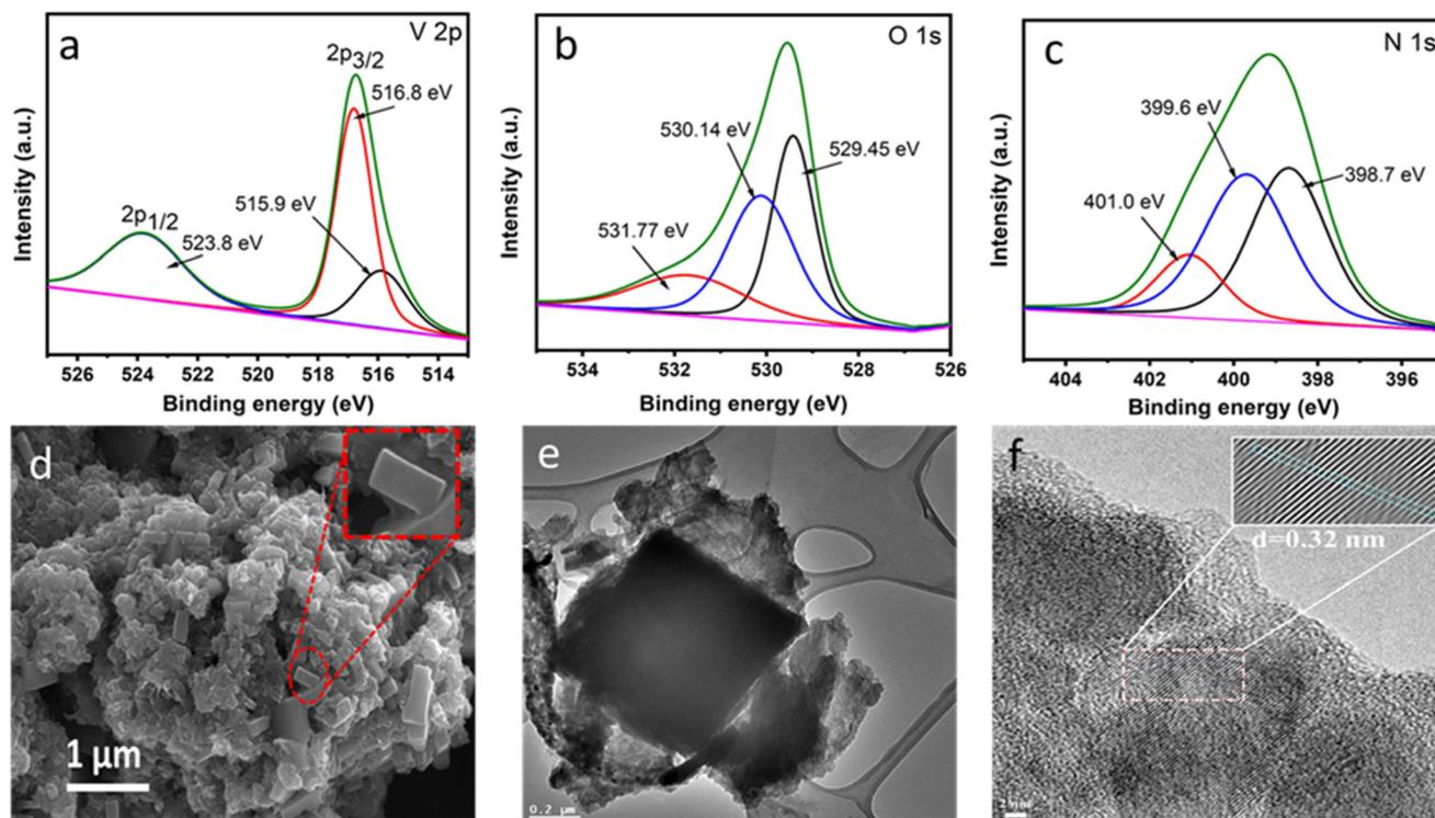
Fig. 3 XPS spectra of  $\text{VO}_2\text{@CN}$ : (a) V 2p, (b) O 1s and (c) N 1s. (d) FESEM image of  $\text{VO}_2\text{@CN}$  indicating the presence of blocks of  $\text{VO}_2$  encapsulated in crumpled N-doped C layers. TEM and HRTEM images of  $\text{VO}_2\text{@CN}$  are presented as (e) and (f), respectively.
