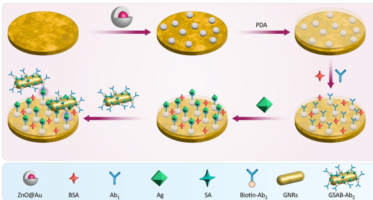
**Fig. 13** The scheme illustrates the assembly of a SPR biosensor, starting with a ZnO@Au nanocomposite base layer. Bovine serum albumin (BSA) and primary antibodies (Ab1) are applied to capture Ag, followed by SA and biotin-Ab<sub>2</sub> to enhance the signal. GNRs and GSAB-Ab<sub>2</sub> are then introduced for signal amplification, creating a sensitive, sandwich-type biosensor for detecting hIgG. Reproduced from ref. 199 with permission from [Elsevier], copyright [2022].
