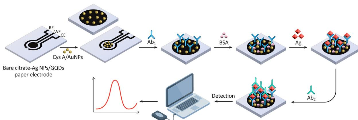
**Fig. 17** This illustration shows the steps for fabricating a paper-based electrochemical biosensor. It begins with a bare electrode modified with AgNPs and GQDs, followed by Ab immobilization, blocking with BSA to prevent non-specific binding, Ag capture, and finally, detection with a secondary antibody (Ab<sub>2</sub>), leading to signal generation for analysis. Reproduced from ref. 222. with permission from [Elsevier], copyright [2020].
