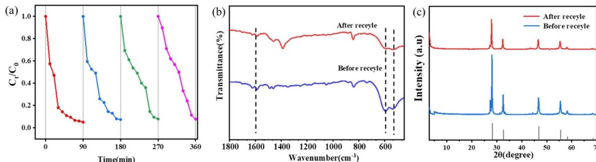
Fig. 6 (a) 1COF : 9BiO<sub>2-x</sub> catalysed by visible light for 4 cycles and FT-IR spectra (b) and XRD patterns (c) of 1COF : 9BiO<sub>2-x</sub> obtained before and after the reaction.
