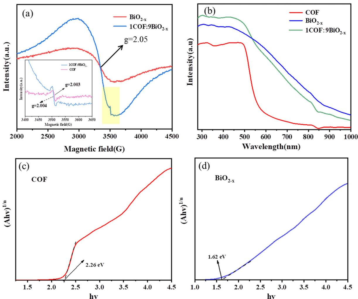
Fig. 4 (a) EPR spectra of  $\text{BiO}_{2-x}$ , the COF and the 1COF:9 $\text{BiO}_{2-x}$  catalyst; (b) UV-vis absorption spectra of the COF,  $\text{BiO}_{2-x}$  and the 1COF:9  $\text{BiO}_{2-x}$  composite; and (c and d) energy band gaps of the COF and  $\text{BiO}_{2-x}$ .
