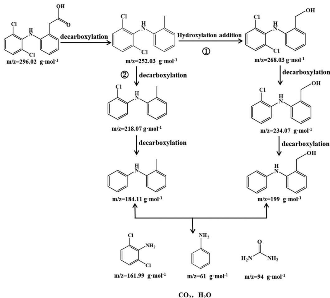
**Scheme 2** The probable degradation mechanism for diclofenac degradation.
