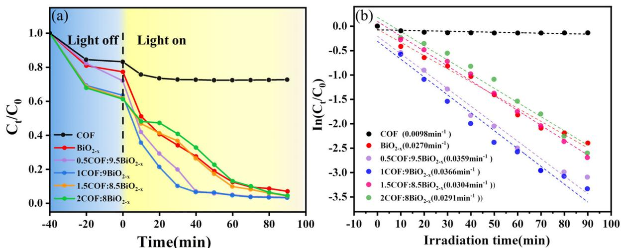
Fig. 5 (a) Photocatalytic degradation of DCF by  $\text{BiO}_{2-x}$  with composites of different weights; (b) DCF rate constant diagram of the photocatalytic degradation of  $\text{BiO}_{2-x}$  with composites of different weights.
