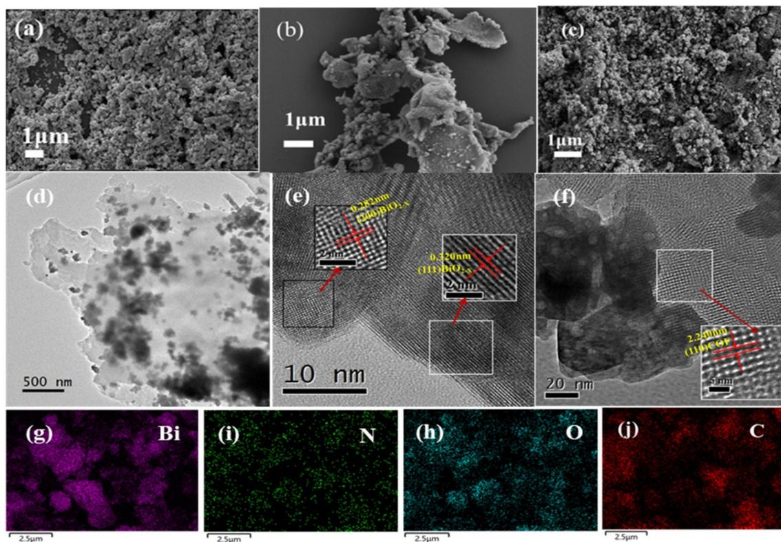
**Fig. 2** SEM images of (a)  $\text{BiO}_{2-x}$ , (b) COF, and (c) 1COF:9 $\text{BiO}_{2-x}$ ; (d) TEM image of the 1COF:9 $\text{BiO}_{2-x}$  sample; (e and f) HRTEM image of 1COF:9 $\text{BiO}_{2-x}$ ; and (g)–(j) mapping images of 1COF:9 $\text{BiO}_{2-x}$ .
