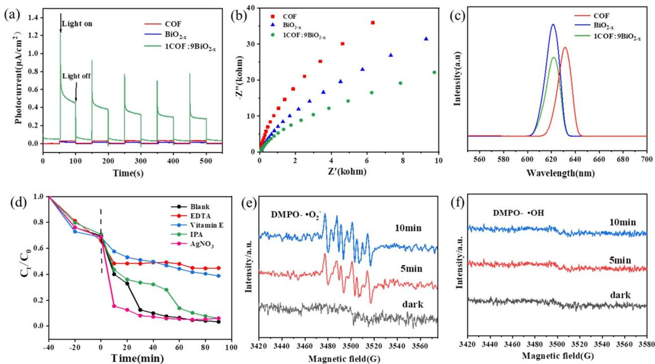
Fig. 7 (a) Transient photocurrent responses, (b) EIS Nyquist plots and (c) PL spectra of the COF,  $\text{BiO}_{2-x}$  and  $1\text{COF}:9\text{BiO}_{2-x}$ ; (d) radical capture experiment; and EPR diagrams of  $1\text{COF}:9\text{BiO}_{2-x}$  DMPO- $\cdot\text{O}_2^-$  (e) and DMPO- $\cdot\text{OH}$  (f) under visible light irradiation.
