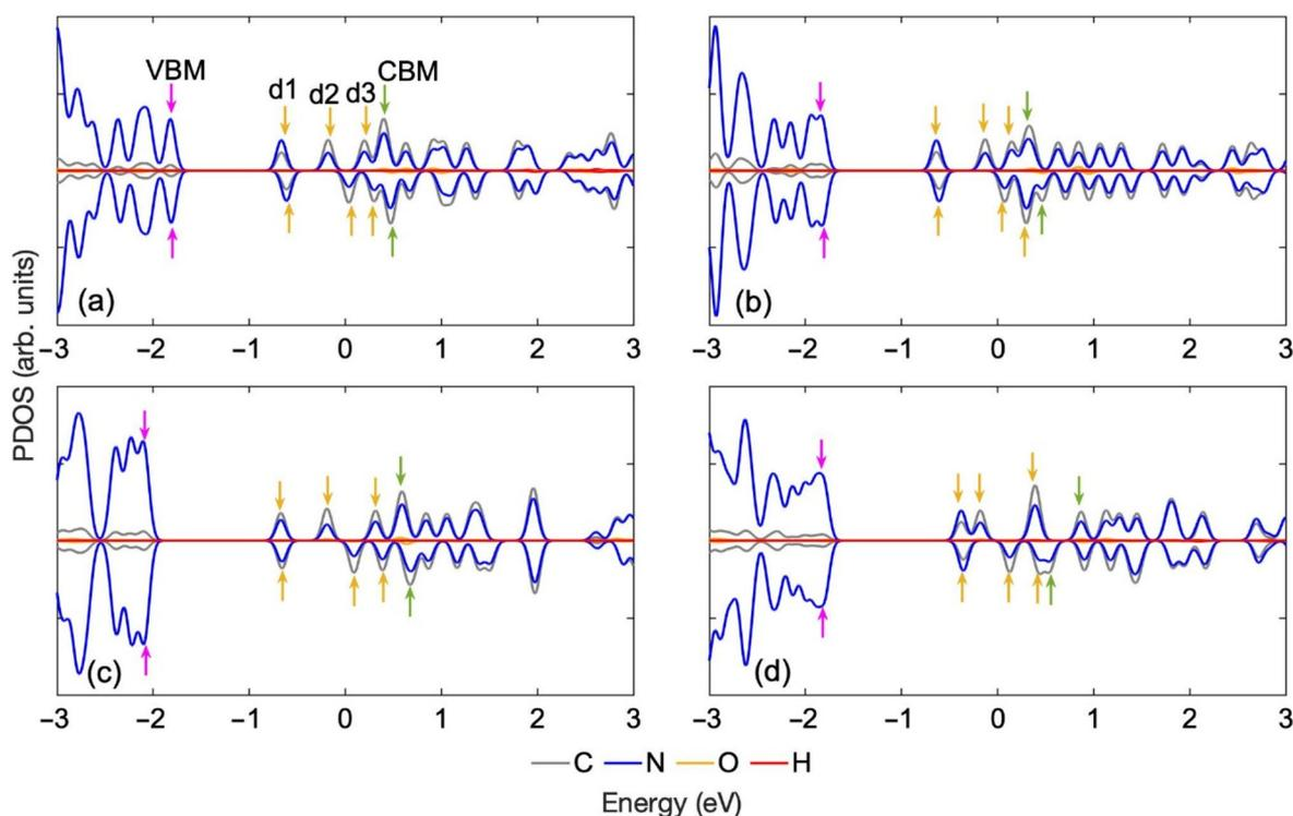
**Fig. 2** Partial density of states (PDOS) for the optimized structures of the ON-GCN tautomers shown in Fig. 1: (a) NH-CN, (b) NH<sub>3</sub>, (c) N-H $\beta$  and (d) N-H $\alpha$ . Hopping of just one hydrogen leads to substantial changes in the electronic properties. The Fermi level is set to 0 eV. Band edges and defect states are marked with colored arrows: VBM: pink, CBM: green, defects (d1–d3): yellow.
