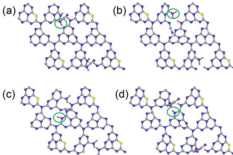
**Fig. 1** Optimized structures of dual defect ON-GCN tautomers. The structures are labeled based on the position of the circled hydrogen atoms as (a) NH–CN (most stable structure), (b) NH<sub>3</sub>, (c) N\_H $\beta$  and (d) N\_H $\alpha$  (least stable structure), Table 1. C: grey, N: blue, O: golden and H: red.
