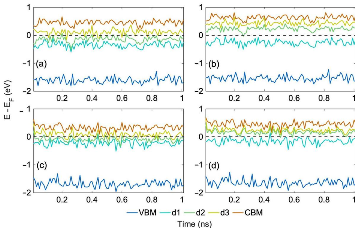
**Fig. 3** (a) Spin up and (b) spin down *ab initio* energy levels calculated every 10 ps along the 1 ns ML trajectory at 300 K starting from the most stable NH-CN structure, Fig. 1a, and (c) spin up, (d) spin down levels for the trajectory starting from the least stable N<sub>H</sub>α structure (Fig. 1d). The corresponding hydrogen hopping trajectories are shown in Fig. 4a and b, respectively. The Fermi energy has been subtracted from the KS state energies to set the Fermi level to 0.
