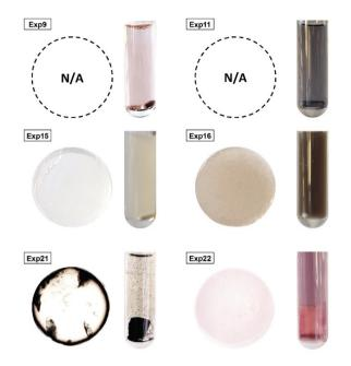
Fig. 4 Experiments identified as outliers showcasing a cross-sectional view of the hydrogels (if formed, which was not the case for Exp 9 and Exp 11) alongside a photograph of the microwave reaction vessel. Reaction conditions can be found in Table S1† with the experiment number.
