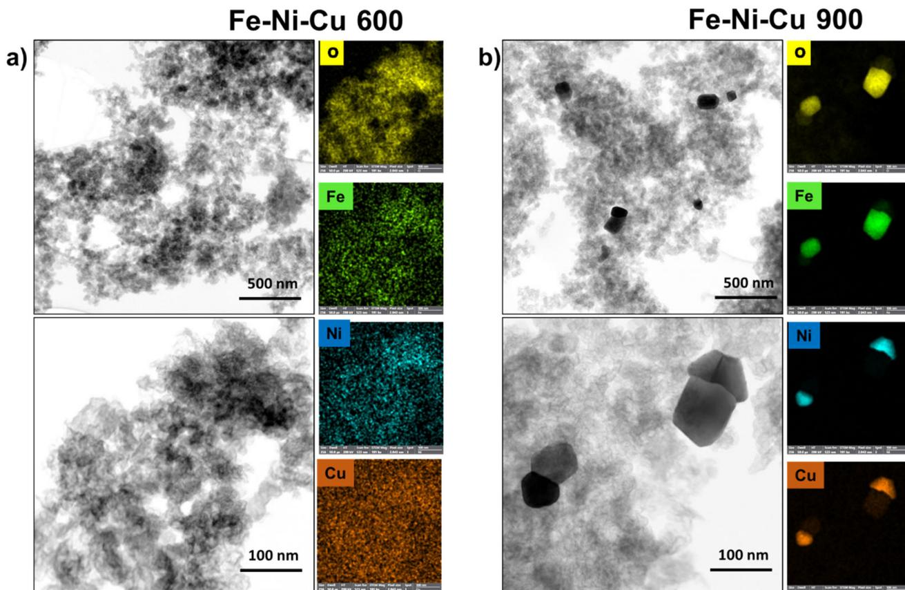
Fig. 3 (a) STEM, and EDX maps at the O, Fe, Ni, Cu K X-ray K of the Fe–Ni–Cu 600 and (b) STEM, and EDX maps at the O, Fe, Ni, Cu X-ray K emissions of the Fe–Ni–Cu 900.
