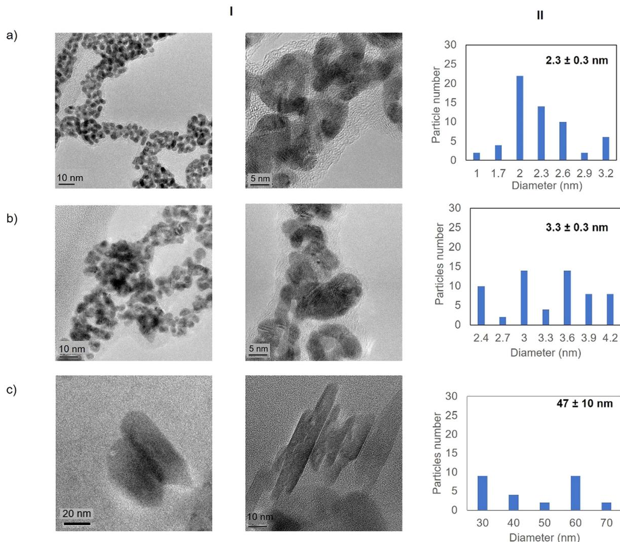
**Fig. 3** Electronic microscopy characterisation of the different GTL-114 gold metalloenzymes. (a) Au-Mt@GTL-114 pH 7, (b) Au-Mt@GTL-114 pH 8.5, (c) Au-Mt@GTL-114 pH 10. (I) TEM and HR-TEM, (II) nanoparticle size distribution graphic.
