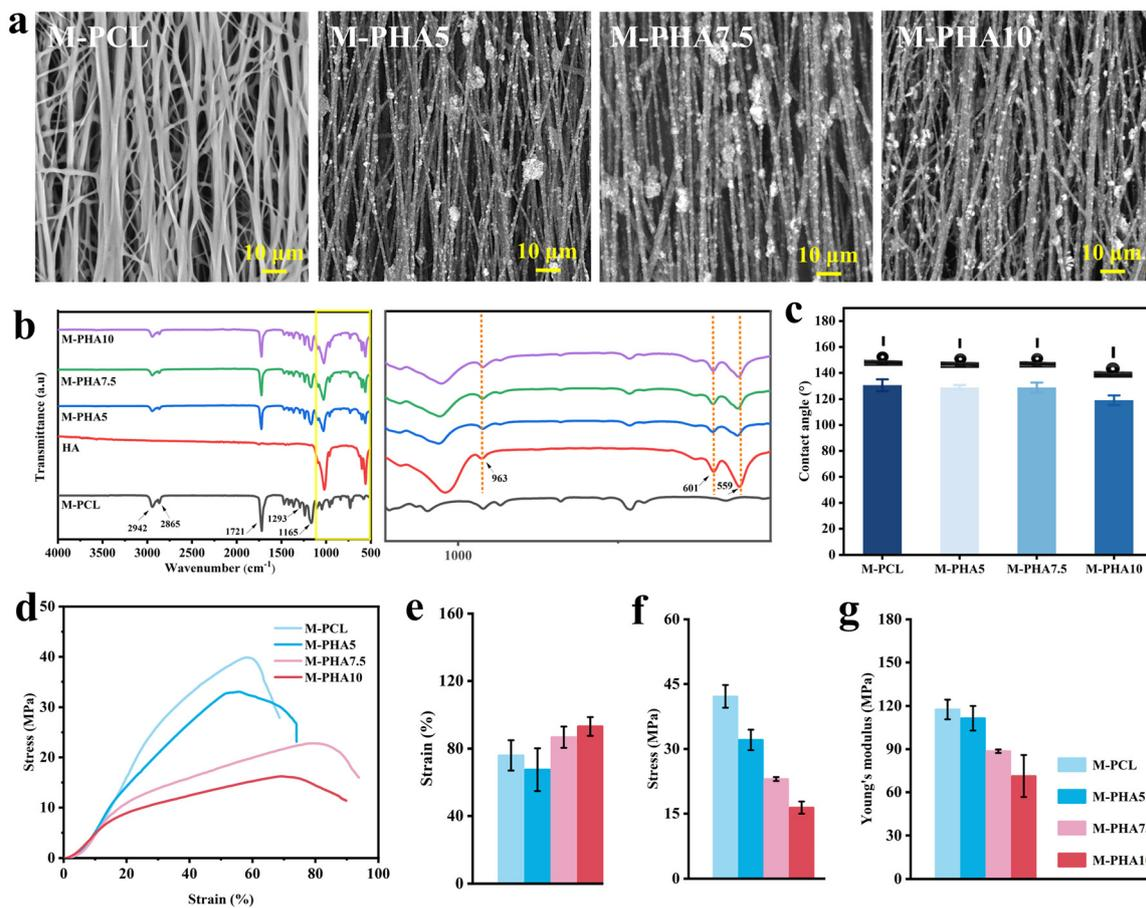
**Fig. 2** Physicochemical characterization of the aligned nanofiber membranes containing different concentrations of n-HA. (a) SEM images; (b) FTIR spectra; (c) measurements of water contact angle; (d) tensile stress–strain curves; and (e–g) the ultimate strain and stress at break and Young's modulus.
