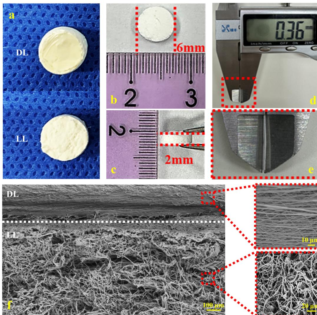
**Fig. 1** Morphological characterization of the composite scaffold. (a) Photograph showing the composite scaffolds. (b and c) The width and thickness of a composite scaffold. (d and e) The thickness of the dense layer. (f) SEM images of the P/CS-T-PHA5 composite scaffold cross-section and the magnified images.
