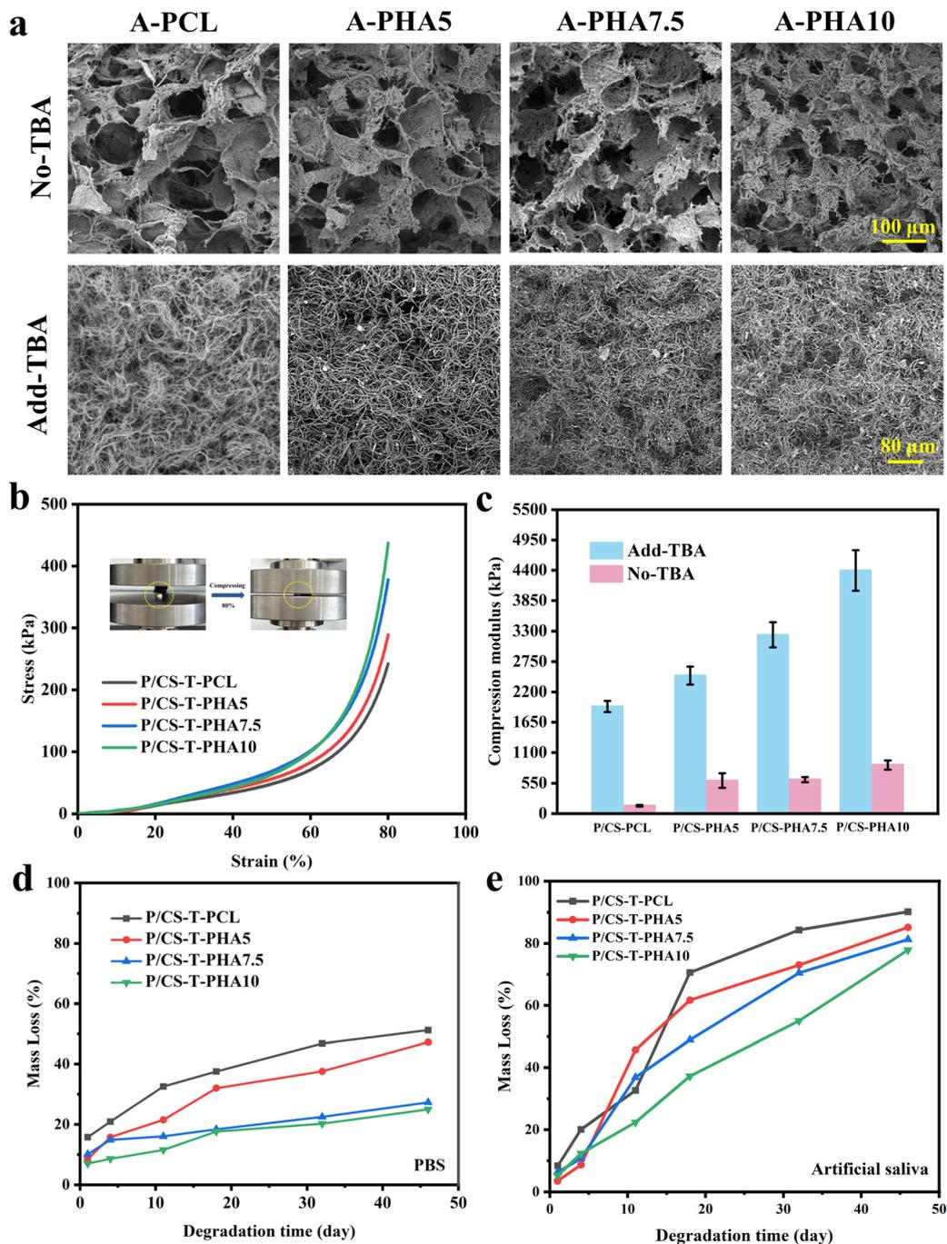
**Fig. 4** (a) SEM images showing the structure of aerogels treated with or without TBA. (b) Compressive stress–strain curves of the composite scaffolds that were treated with TBA and contained different n-HA contents. (c) Compression modulus of the composite scaffolds treated with and without TBA. (d and e) Mass loss during the biodegradation of different composite scaffolds in (d) PBS and (e) artificial saliva.
