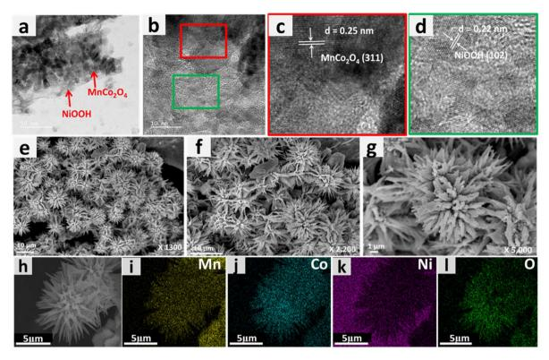
Fig. 5 (a) TEM image after the durability test. (b), (c) and (d) HRTEM images after the durability test confirming the presence of (c)  $MnCo_2O_4$  and (d) NiOOH. (e-g) FESEM images of  $MnCo_2O_4$ -NiOOH after the durability test. (h-l) FESEM elemental mapping of the catalyst after the durability test.
