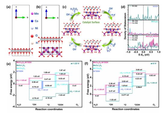
Fig. 6 Theoretical models of (a)  $MnCo_2O_4$  and (b)  $MnCo_2O_4$ -NiOOH. (c) illustration of the mechanism for the OER on the heterostructure(d) Projected orbital DOS plot. Gibbs free energy plot for the OER (e) at 1.23 V and (f) at 0 V for  $MnCo_2O_4$ , NiOOH, and  $MnCo_2O_4$ -NiOOH.
