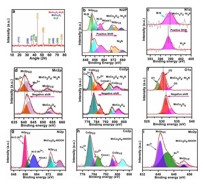
Fig. 1 (a) PXRD pattern of MnCo<sub>2</sub>O<sub>4</sub>-Ni<sub>3</sub>N. High-resolution (b) Ni2p present in MnCo<sub>2</sub>O<sub>4</sub>-Ni<sub>3</sub>N and Ni<sub>3</sub>N. (c) N1s present in MnCo<sub>2</sub>O<sub>4</sub>-Ni<sub>3</sub>N and Ni<sub>3</sub>N. (d) Mn2p, (e) Co2p and (f) O1s present in MnCo<sub>2</sub>O<sub>4</sub>-Ni<sub>3</sub>N and MnCo<sub>2</sub>O<sub>4</sub>. (g) Ni2p (h) Co2p and (i) Mn2p XPS spectra of MnCo<sub>2</sub>O<sub>4</sub>-NiOOH.
