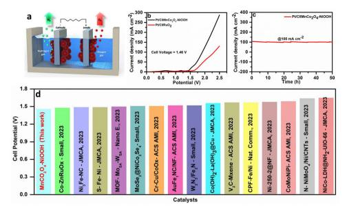
Fig. 7 (a) Schematic representation of the cell for overall water splitting. (b) LSV curve in two-electrode setup. (c) Durability test using chronoam-perometry. (d) Comparison of cell potential with the cell potentials of recently reported catalysts.
