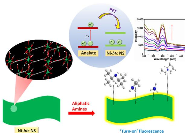
Scheme 2 Schematic illustration of the aliphatic amine sensing by Ni-*btc* NS.
