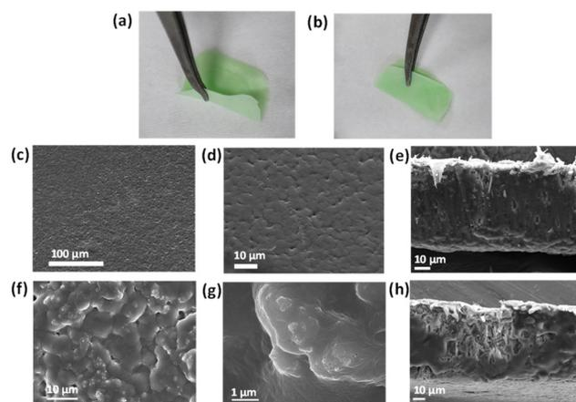
**Fig. 4** (a and b) Elucidating the flexibility of membrane; (c) and (d) FESEM images of the PVDF membrane indicating smooth surface; (e) FESEM image of the cross-section of PVDF membrane; (f and g) FESEM images of Ni-btc NS MMM showing MOF NS embedded in membrane and (h) FESEM image of the cross-section of Ni-btc NS MMM.
