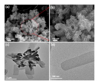
Fig. 1 (a) FESEM image of NiO NS showing nanosheets agglomerated to form nanoflower morphology. (b) Magnified FESEM image of NiO NS. (c) TEM image of Ni-btc NS showing aggregated nanosheets and (d) TEM image of the single nanosheet of Ni-btc NS at a higher magnification.
