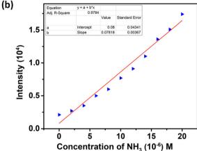
Fig. 2 (a) Emission spectrum of Ni-btc NS dispersed in water showing increase in intensity upon gradual addition of ammonia solution. (b) Determination of LOD via linear fitting of the fluorescence intensity of Ni-btc NS upon adding different concentrations of ammonia solution at  $\lambda_{\text{emi}}$  = 400 nm (upon  $\lambda_{\text{exc}}$  = 310 nm).
