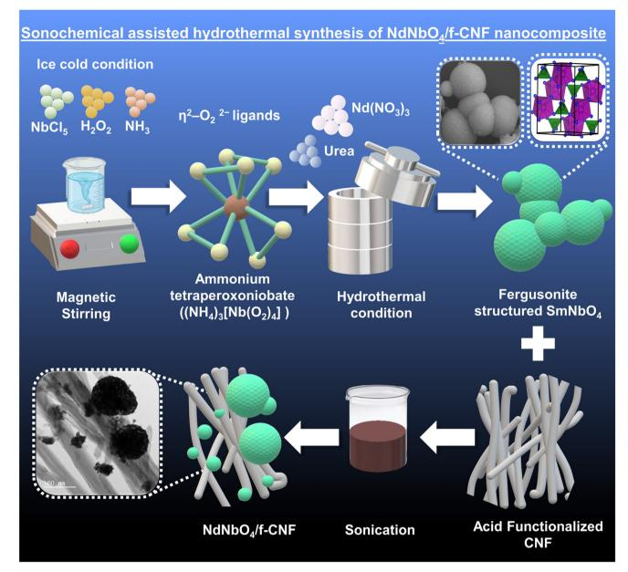
Fig. 1 Schematic representation of the synthesis of the NdNbO<sub>4</sub> reinforced f-CNF nanocomposite.
