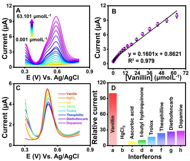
Fig. 6 (A) DPV curves obtained using NdNbO<sub>4</sub>/f-CNF/GCE with a sequential increase in the VAN concentration; (B) corresponding linear dependence plot of VAN concentration *versus* anodic peak currents; (C) DPV profile for  $100 \mu mol L^{-1}$  VAN at NdNbO<sub>4</sub>/f-CNF/GCE in the presence of overlapping agents at the anodic scan; and (D) relative current error percentage obtained by each interferon with respect to the anodic peak current of VAN.
