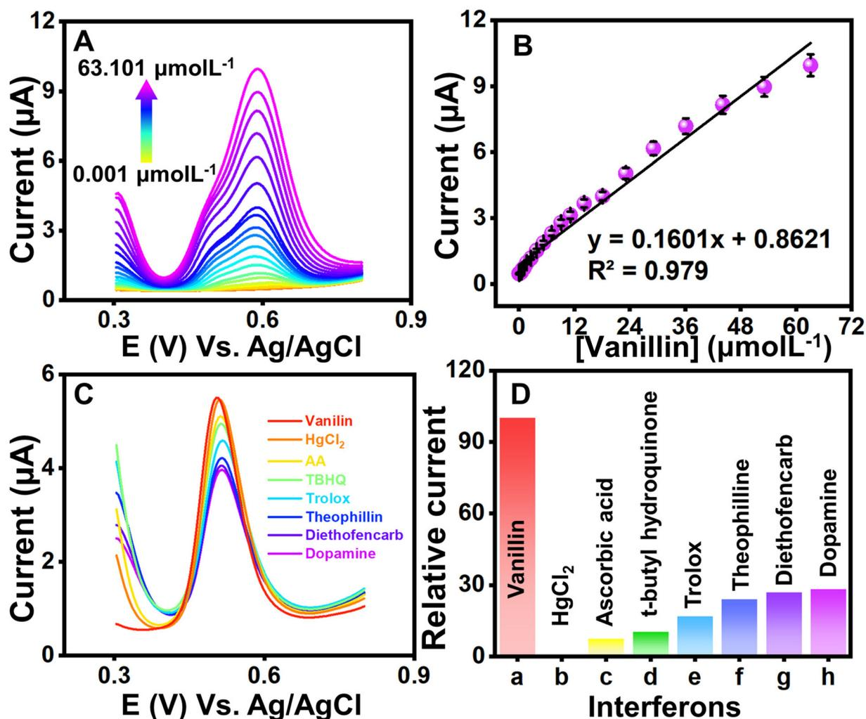
**Fig. 6** (A) DPV curves obtained using NdNbO<sub>4</sub>/f-CNF/GCE with a sequential increase in the VAN concentration; (B) corresponding linear dependence plot of VAN concentration versus anodic peak currents; (C) DPV profile for 100  $\mu\text{mol L}^{-1}$  VAN at NdNbO<sub>4</sub>/f-CNF/GCE in the presence of overlapping agents at the anodic scan; and (D) relative current error percentage obtained by each interferon with respect to the anodic peak current of VAN.
