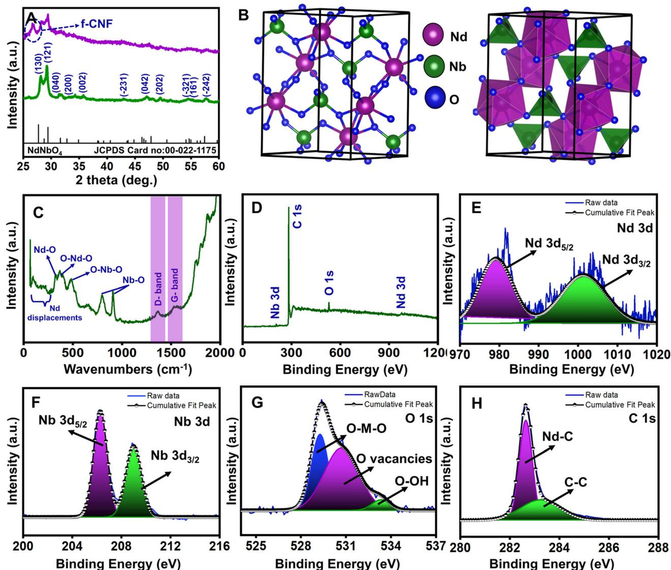
Fig. 2 (A) X-ray diffraction patterns of pure NdNbO<sub>4</sub> and the NdNbO<sub>4</sub>/f-CNF nanocomposite; (B) crystal structure of NdNbO<sub>4</sub> nanocrystallites; (C) Raman spectra of the NdNbO<sub>4</sub>/f-CNF nanocomposite; (D) XPS survey spectra of the NdNbO<sub>4</sub>/f-CNF nanocomposite; and high-resolution XPS spectra of (E) Nd 3d, (F) Nb 3d, (G) O 1s and (H) C 1s.
