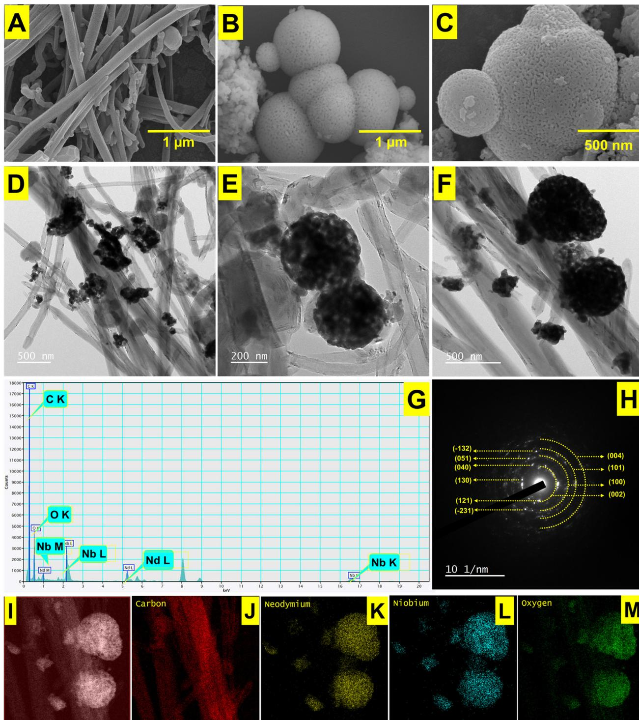
**Fig. 3** FESEM micrographs of (A) f-CNF and (B and C) NdNbO<sub>4</sub>; (D–F) TEM images, (G) EDX spectrum, (H) SAED pattern, and (I–M) elemental mapping of the NdNbO<sub>4</sub>/f-CNF nanocomposite.
