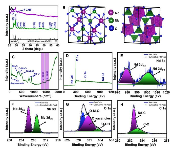
Fig. 2 (A) X-ray diffraction patterns of pure  $NdNbO_4$  and the  $NdNbO_4/f$ -CNF nanocomposite; (B) crystal structure of  $NdNbO_4$  nanocrystallites; (C) Raman spectra of the  $NdNbO_4/f$ -CNF nanocomposite; and high-resolution XPS spectra of (E) Nd 3d, (F) Nb 3d, (G) O 1s and (H) C 1s.
