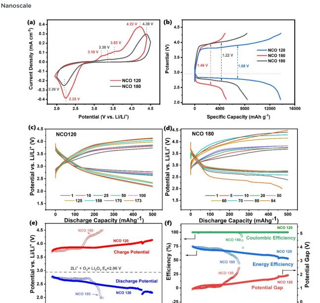
Fig. 4 (a) CV analysis @0.2 mV s $^{-1}$  and (b) full discharge—charge @100 mA g $^{-1}$ , and selected discharge—charge curves of (c) NCO 120 and (d) NCO 180 cathode-based LABs operated at 100 mA g $^{-1}$  for a limited capacity of 500 mA h g $^{-1}$ . (e and f) Cycle life and performance analysis of LABs with NCO 120 and NCO 180 based cathodes with cut-off discharge capacity of 500 mA h g $^{-1}$  with 1 M LiTFSI dissolved in TEGDME electrolyte.
