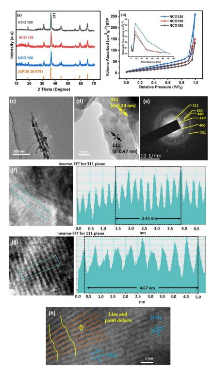
Fig. 2 (a) XRD patterns of the synthesized NiCo<sub>2</sub>O<sub>4</sub> structures on Ni foam, (b) nitrogen adsorption/desorption isotherms and pore size distribution curve of NiCo<sub>2</sub>O<sub>4</sub> structures, (c) TEM image, (d) HRTEM image, (e) corresponding SAED pattern, (f and g) inverse-FFT analysis for the NCO 120 structure, and (h) crystal defects.
