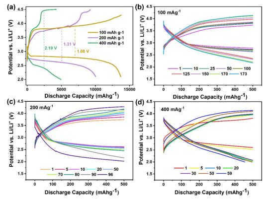
Fig. 5 Electrochemical performance analysis of NCO 120 cathode-based LABs under different current densities: (a) full discharge-charge capacity, selected discharge-charge curves under a current density of (b) 100 mA  $g^{-1}$ , (c) 200 mA  $g^{-1}$ , and (d) 400 mA  $g^{-1}$ .
