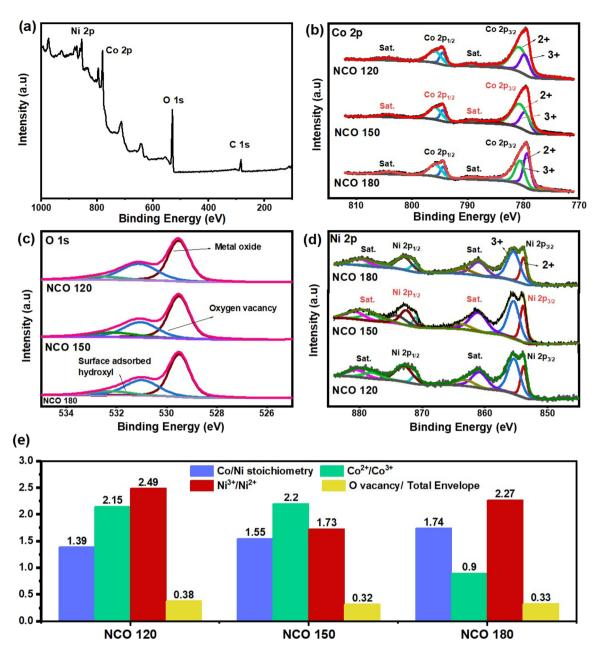
Fig. 3 XPS analysis: (a) survey spectrum, (b) Co 2p spectra, (c) O 1s spectra, (d) Ni 2p spectra of as-synthesized NiCo<sub>2</sub>O<sub>4</sub> catalysts on Ni foam, and (e) extrapolated co-relations *via* peak area analysis.
