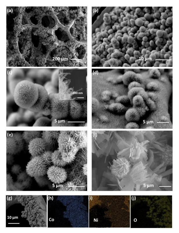
Fig. 1 SEM images of different Ni-Co oxide structures anchored on Ni foam, (a-d) low and high magnifications of the NCO 120 structure, (e) NCO 150, (f) NCO 180, and (g-j) EDX analysis of the NCO 120 structure.
