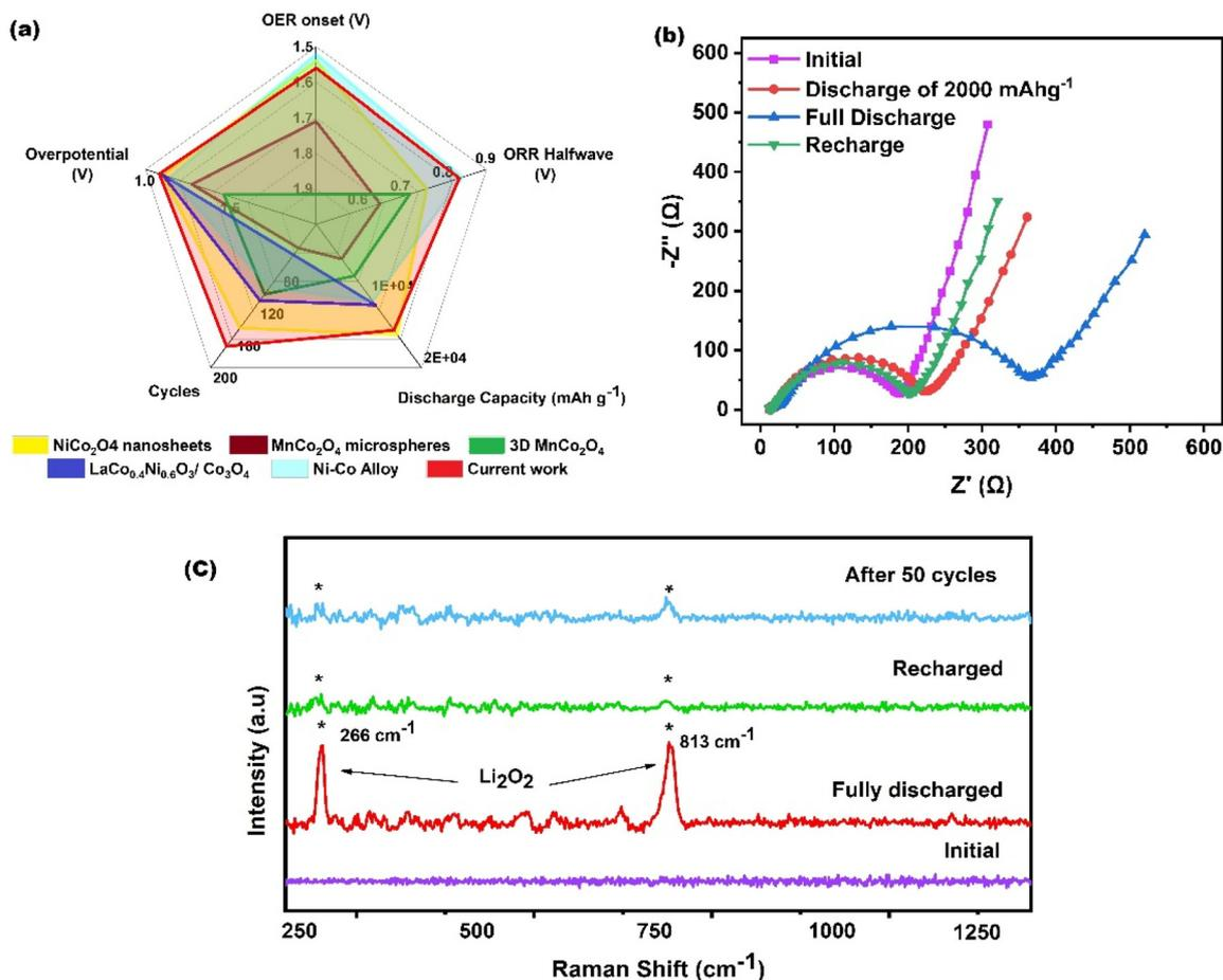
**Fig. 6** (a) Literature comparison,<sup>41–45</sup> (b) EIS analysis, (c) *ex situ* Raman analysis of LAB cells with the freestanding NCO 120 cathode at various levels of discharge and charge.
