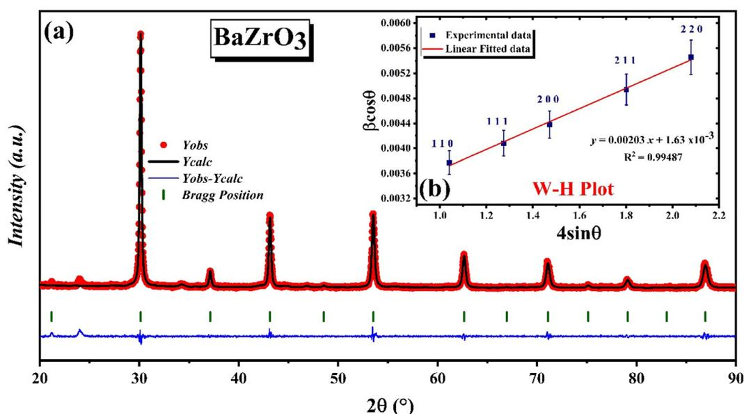
Fig. 3 (a) Rietveld refined X-ray diffraction pattern of BaZrO<sub>3</sub> nanoparticle and (b) W–H plot.
