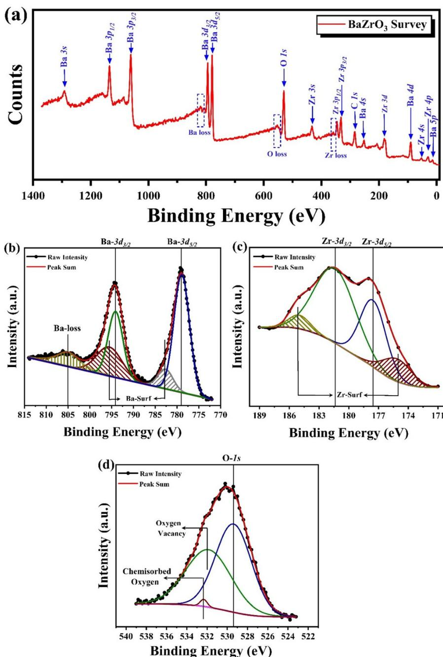
Fig. 7 (a) XPS survey spectra of BaZrO<sub>3</sub> nanoparticles (b) XPS spectra of Ba-3d element, (c) XPS spectra of Zr-3d element, and (d) XPS spectra of O-1s element.
