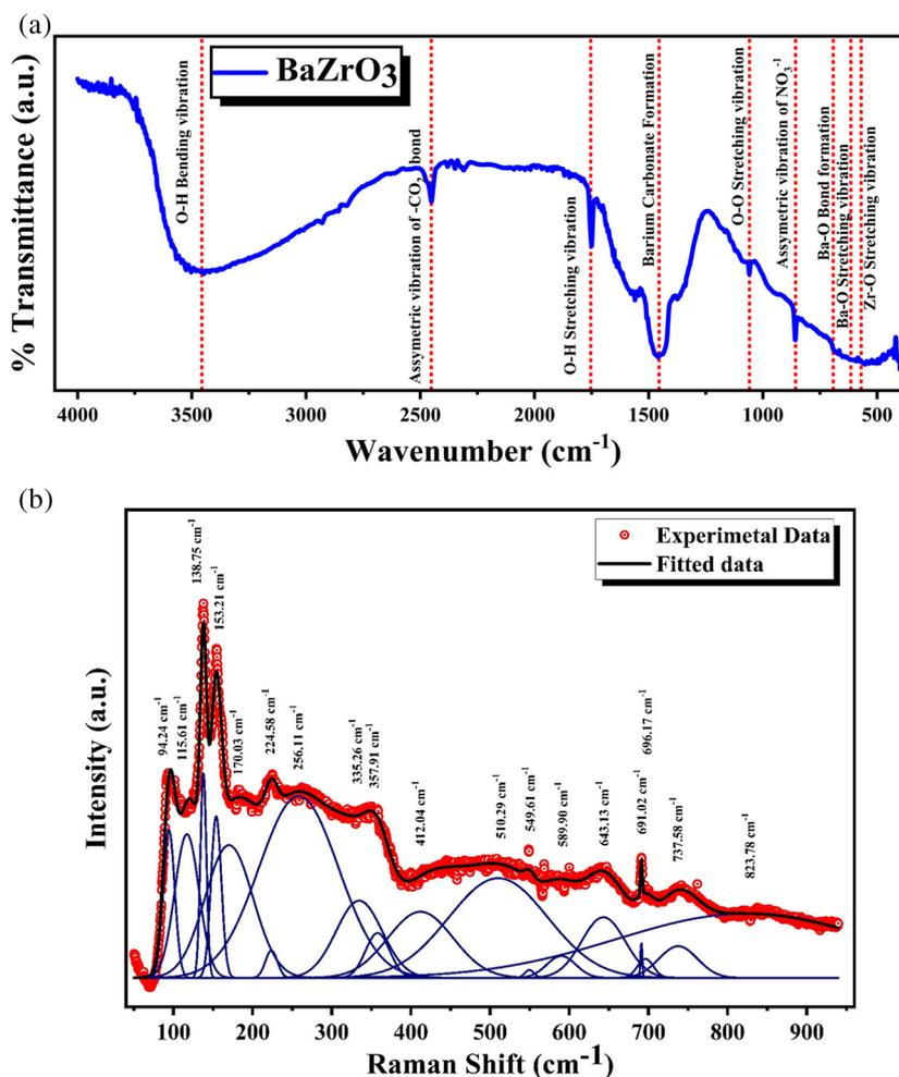
Fig. 6 (a) FT-IR spectra of BaZrO<sub>3</sub>. (b). Room temperature Raman spectra of BaZrO<sub>3</sub> nanoparticles.
