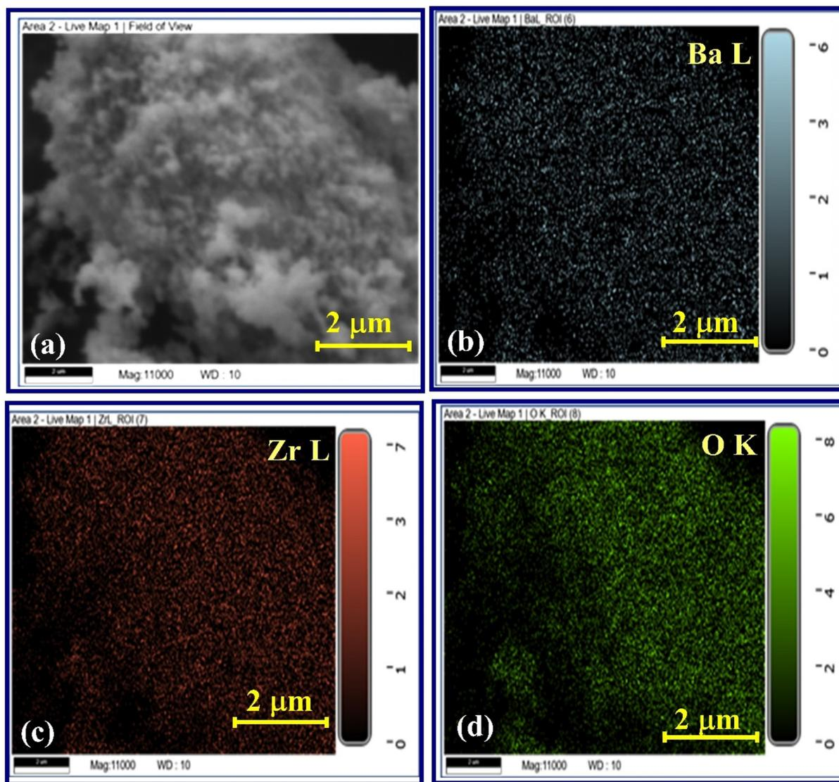
Fig. 5 (a) Field of view for EDS mapping, (b) EDS mapping for Ba L, (c) EDS mapping for Zr L and (d) EDS mapping of O K elements of BaZrO<sub>3</sub> nanoparticles.
