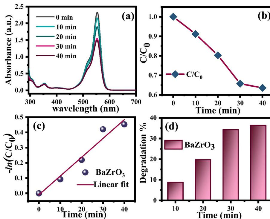
**Fig. 9** (a) Degradation absorbance spectra of RhB dye using BaZrO<sub>3</sub> nanoparticles, and (b) and (c) degradation rate. (d) Efficiency of dye for degradation under visible light.
