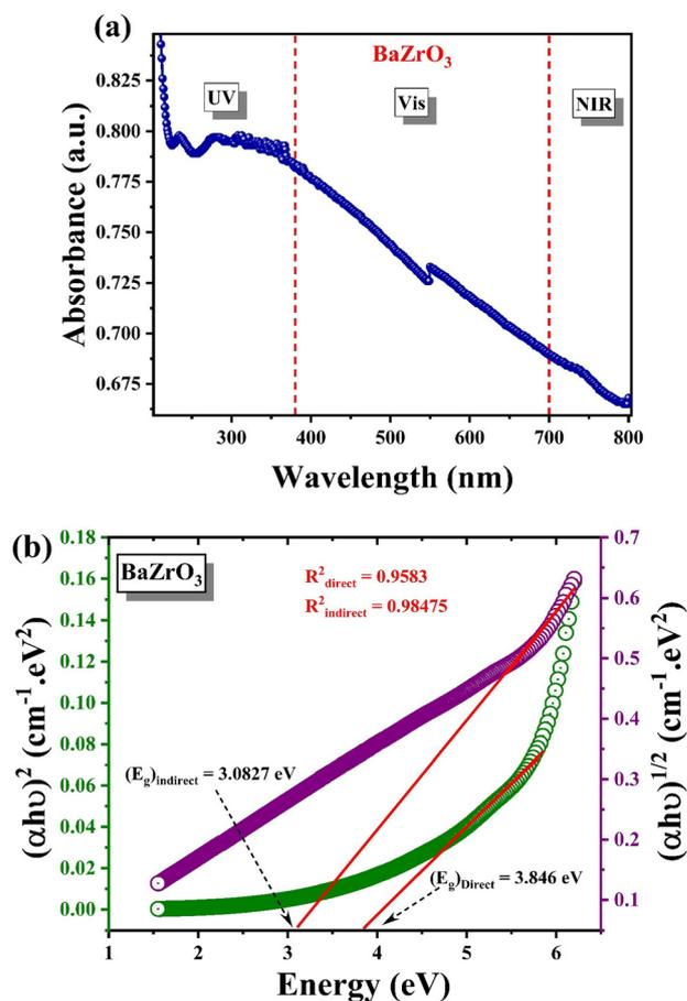
**Fig. 8** (a) UV-Vis spectra of BaZrO<sub>3</sub>. (b) Tauc plot of BaZrO<sub>3</sub> nanoparticles.
