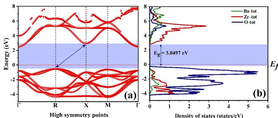
Fig. 10 (a) Electronic band structure, (b) total density of states of BaZrO<sub>3</sub> nanoparticle.
