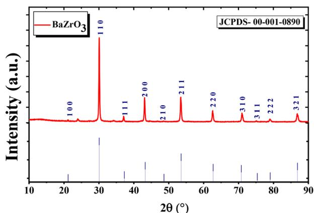
Fig. 2 XRD patterns of the as-synthesized BaZrO<sub>3</sub> nanoparticles.
