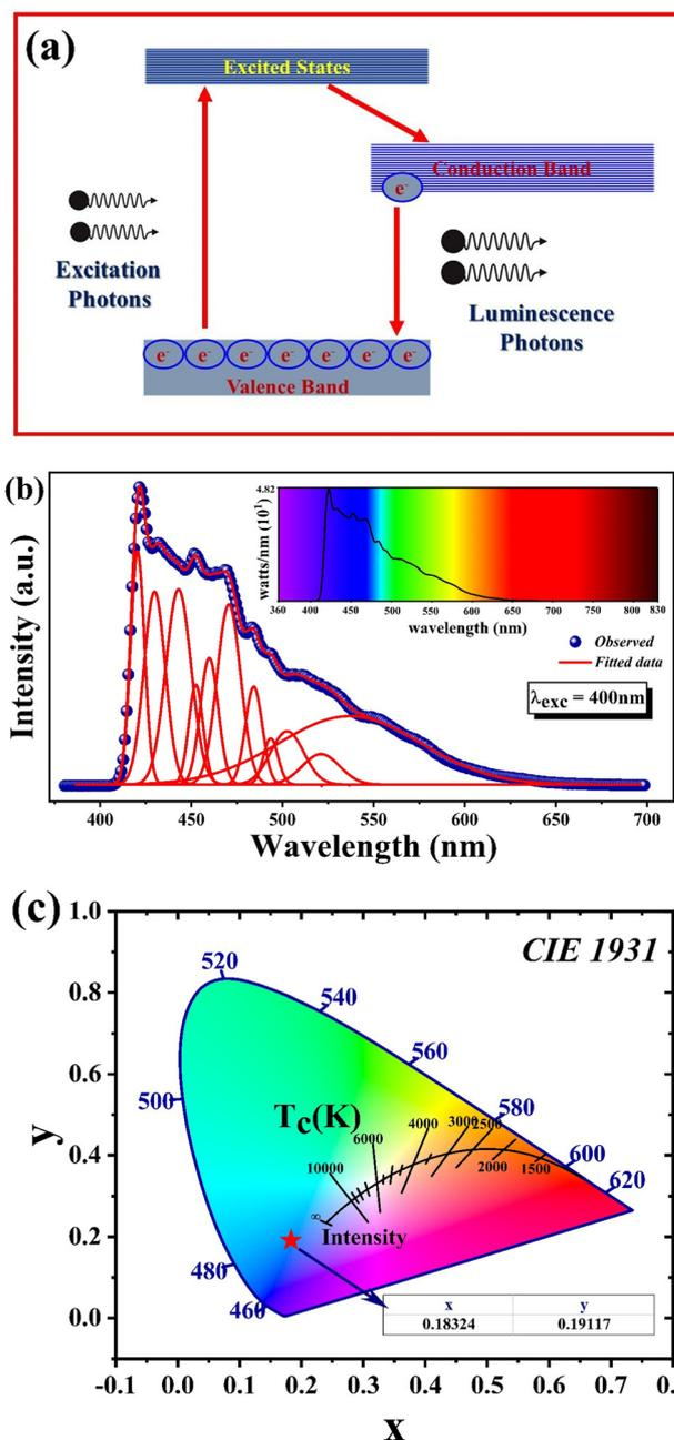
Fig. 11 (a) Photoluminescence mechanism. (b) Photo luminescence spectra at the excitation wavelength  $\lambda_{\text{exc}} = 400$  nm. (c) CIE diagram of BaZrO<sub>3</sub> nanoparticles.
