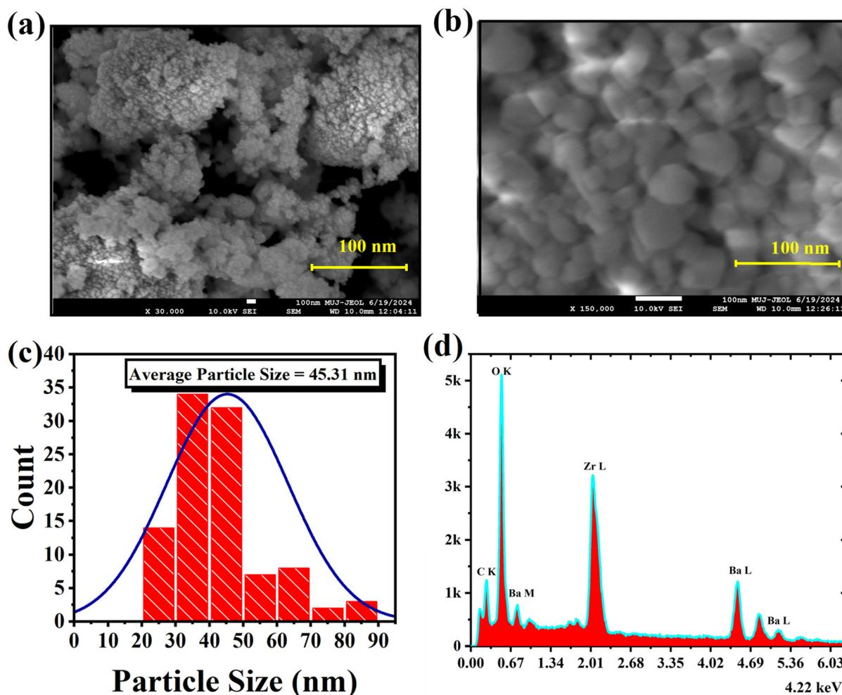
Fig. 4 (a and b) Surface morphology micrographs, (c) average particle size distribution of BaZrO<sub>3</sub>, and (d) EDAX spectra.
