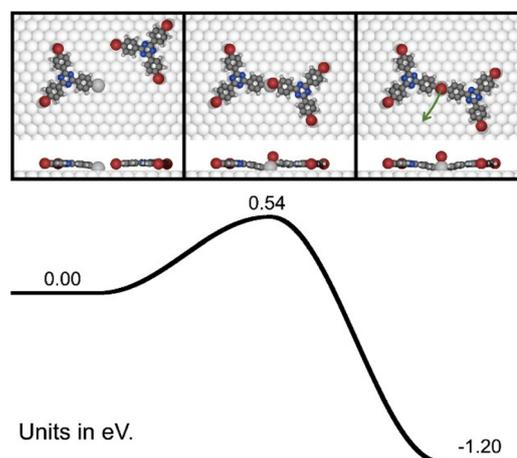
**Fig. 4** DFT calculated energy profile of an alternative debromination reaction on Ag(111) for 3BPT. Thereby, the immobilized organometallic Ag atom from a preceding debromination reaction acts as active site. This process exhibits an even lower activation energy and a markedly increased exothermic reaction energy. The final state energy of the debromination was evaluated with the bromine atom adsorbed on Ag(111), but isolated from the molecular structure.
