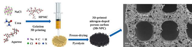
**Fig. 7** Schematic for the fabrication of 3D nitrogen-doped porous carbon by DIW and the resulting morphology.<sup>70</sup>
