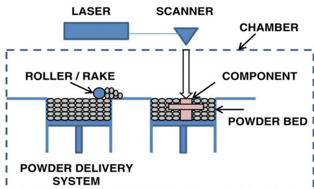
Fig. 4 Schematic of powder bed fusion.<sup>60</sup>
