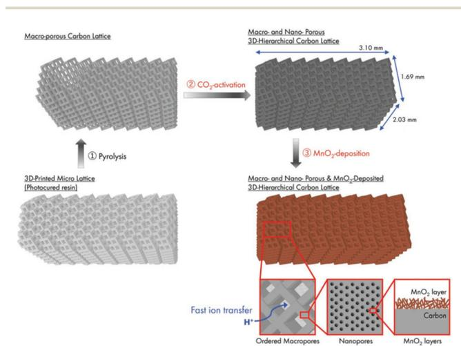
Fig. 10 Schematic of the process for the preparation of a 3D-printed hierarchical porous carbon lattice with  $\text{MnO}_2$  deposition.<sup>82</sup>
