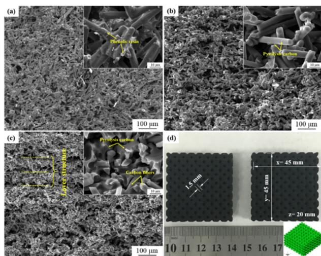
**Fig. 15** SEM images of (a) the SLS green part, cross-section of (b) the carbonized part and (c) the carbon fiber/C preform; (d) picture of complex green parts with lattice structures. The insets are zoom-in SEM images.<sup>95</sup>
