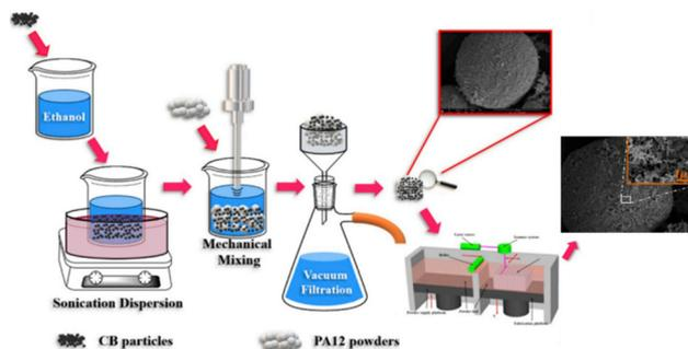
Fig. 13 Schematic illustration of the two-step approach for producing carbon black/polyamide 12 composites with a 3D segregated conductive network.<sup>93</sup>
