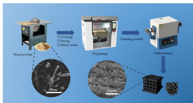
Fig. 12 Schematic diagram of pine resin porous carbon electrode preparation by SLS.<sup>92</sup>
