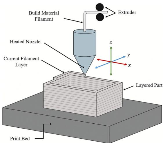
Fig. 2 The basic working principle of material extrusion printing.<sup>44</sup>
