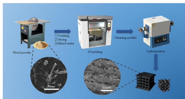
Fig. 12 Schematic diagram of pine resin porous carbon electrode preparation by SLS. 92
