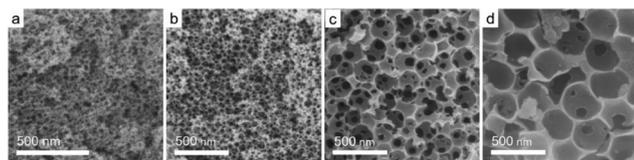
**Fig. 6** SEM of the printed carbon replicas with different SiO<sub>2</sub> diameters: (a) 50 nm; (b) 100 nm; (c) 200 nm; and (d) 350 nm.<sup>69</sup>
