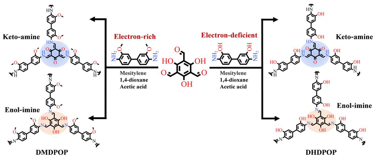
**Scheme 1** Designing POP structures with electron-rich  $\pi$ -electron (*i.e.*, DMDPOP-X) and electron-deficient  $\pi$ -electron (DHDPOP-X) systems.
