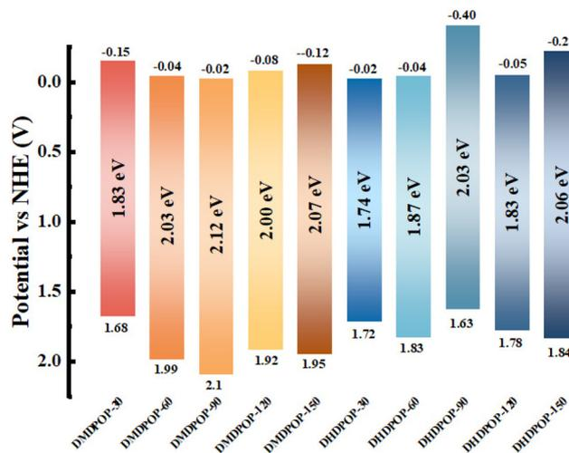
Fig. 6 Calculated band structures of the ten POPs.
