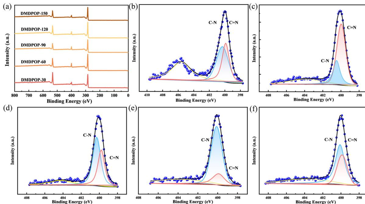
Fig. 3 (a) Full XPS and high-resolution XPS N 1s spectra of DMDPOP-30 (b), DMDPOP-60 (c), DMDPOP-90 (d), DMDPOP-120 (e) and DMDPOP-150 (f).
