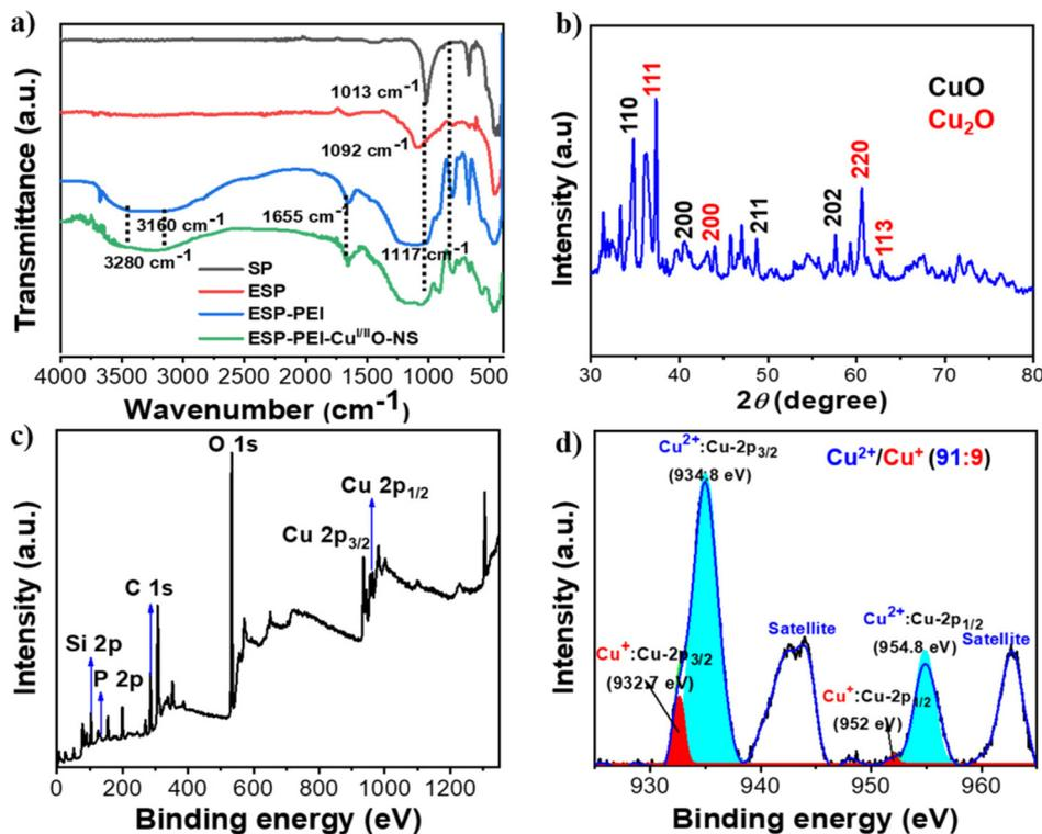
Fig. 1 (a) Overlapped FT-IR spectra of SP, ESP, ESP-PEI, and ESP-PEI-Cu<sup>II</sup>O-NS, (b) PXRD pattern of ESP-PEI-Cu<sup>II</sup>O-NS, (c) XPS spectra of ESP-PEI-Cu<sup>II</sup>O-NS, and (d) high-resolution XPS-survey spectra of Cu<sup>II</sup>O NPs of the copper 2p profile of the ESP-PEI-Cu<sup>II</sup>O-NS catalyst.
