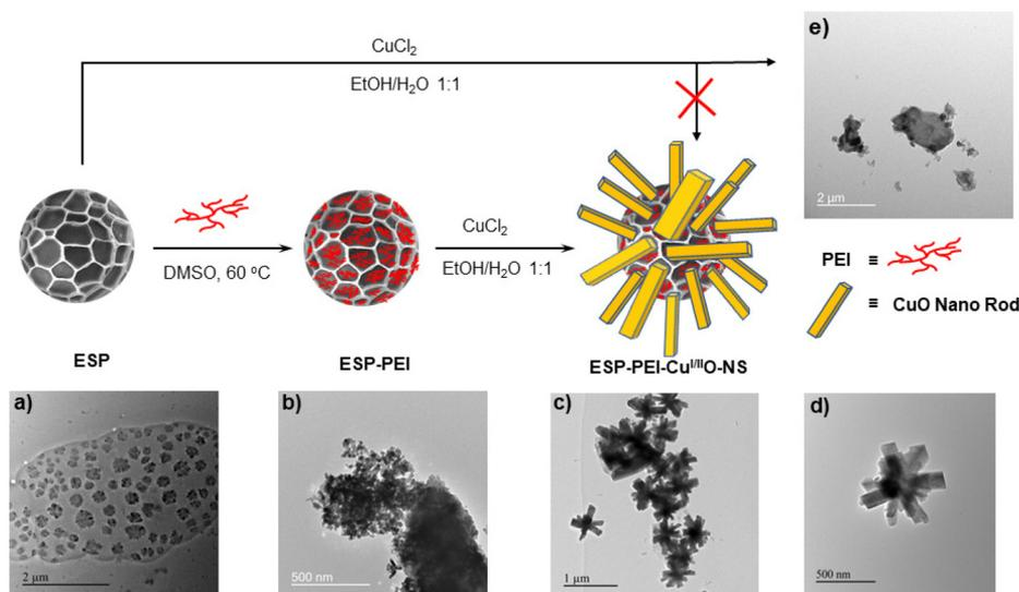
**Scheme 1** Synthetic route to the ESP-templated Cu<sup>II</sup>O nanostar; TEM image of (a) sporopollenin without the genetic material (ESP), (b) PEI coated ESP (ESP-PEI), (c) copper-oxide nanostars (ESP-PEI-Cu<sup>II</sup>O-NS), (d) zoomed image of copper-oxide nanostars (ESP-PEI-Cu<sup>II</sup>O-NS), and (e) PEI-unfunctionalized ESP-Cu<sup>II</sup>O.
