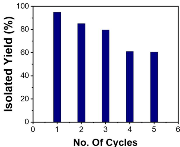
Fig. 2 Isolated yields of 3a using the ESP-PEI-Cu<sup>III</sup>O-NS catalyst up to five cycles.
