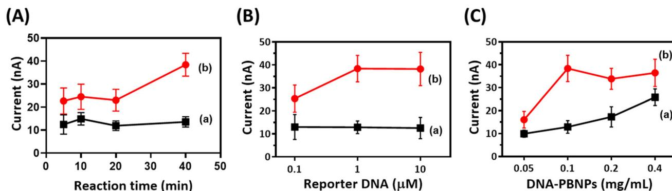
**Fig. 4** Optimization of the DNA-PBNP-based biosensor for  $\text{Cu}^{2+}$  detection. The effect on output signal of the reaction time of  $\text{Cu}^{2+}$ -DNAzyme self-cleavage (A), the concentration of reporter DNA (B) and the concentration of DNA-PBNPs (C).  $N = 3$ , mean  $\pm$  SD.
