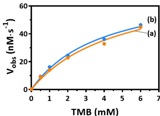
Fig. 2 The catalytic activity of the PBNPs and DNA–PBNPs revealed by the rates of oxidation of TMB<sub>red</sub> to TMB<sub>ox</sub> by PBNPs (a) and DNA–PBNPs (b) in the presence of H<sub>2</sub>O<sub>2</sub>. [H<sub>2</sub>O<sub>2</sub>] = 2 mM, [PBNP] or [DNA–PBNPs] = 10 μg mL<sup>-1</sup>.
