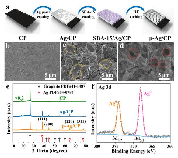
Fig. 1 (a) Schematic diagram of the synthetic process of p-Aq/CP. SEM images of (b) CP, (c) Aq/CP, and (d) p-Aq/CP. (e) XRD patterns of CP, Aq/CP, and p-Ag/CP. (f) High-resolution Ag 3d XPS spectrum of p-Ag/CP.
