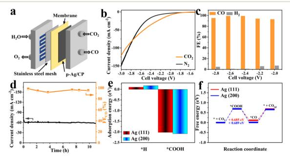
Fig. 4 (a) Schematic configuration of the MEA instrument. (b) LSV curves (10 mV s<sup>-1</sup>) with CO<sub>2</sub>/N<sub>2</sub> supplies. (c) FE<sub>CO</sub> at different applied potentials. (d) Stability test at -2.6 V over 11 h. (e) Calculated adsorption energies of \*H and \*COOH on Ag (111) and (200) surfaces. (f) Calculated free energy profile for the CO<sub>2</sub>RR of p-Ag/CP.
